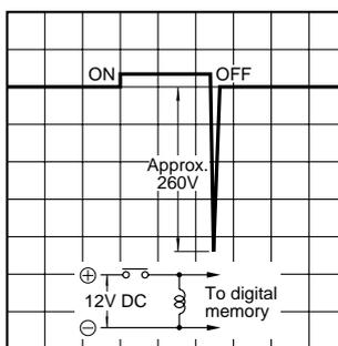
5-(2). DC coil surge voltage waveform (With diode)
