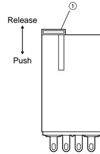
2) To lock to one side turn 90° counter-clockwise while pushing lock and turn 90° clockwise to release.
