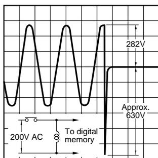
5-(1). DC coil surge voltage waveform (Without diode)
