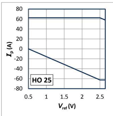
Upper limit:  $I_p = 62.5$  ( $V_{ref} = 0.5 \dots 2.5$  V)
