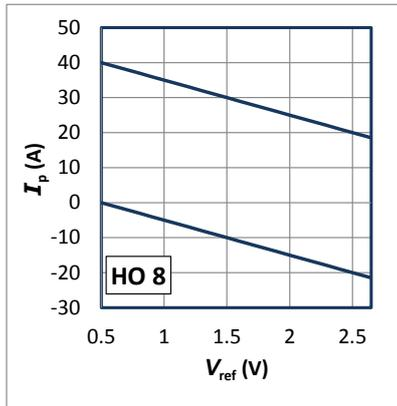
Upper limit:  $I_p = -10 \times V_{ref} + 45$  ( $V_{ref} = 0.5 \dots 2.65$  V)
