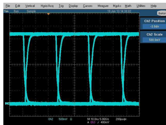
Figure 17. Eye Diagram at 40 Mbps, 2.7V at 25^\circ\text{C}
