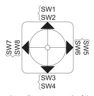
Two switches will actuate in each of the four directions; North, South, East & West.
