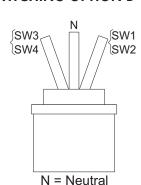
Two switches will actuate as the joystick moves away from centre, in either direction.
