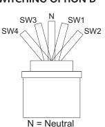
One switch will actuate after 50% of travel, with a further switch at the end of travel, in either direction.
