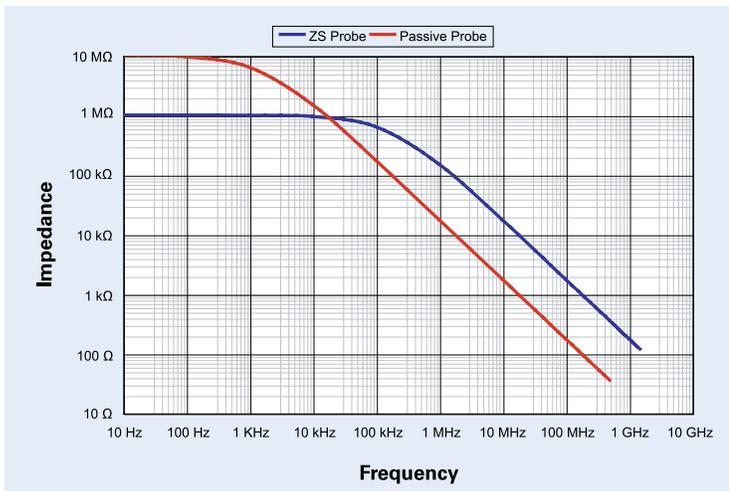
Passive probes are great for low frequency measurements; however, the input capacitance reduces impedance above 1 kHz. The 1 M $\Omega$  input resistance and 0.9 pF capacitance of the ZS probe provide high impedance across the entire probe bandwidth making it the ideal tool for all your probing needs.
