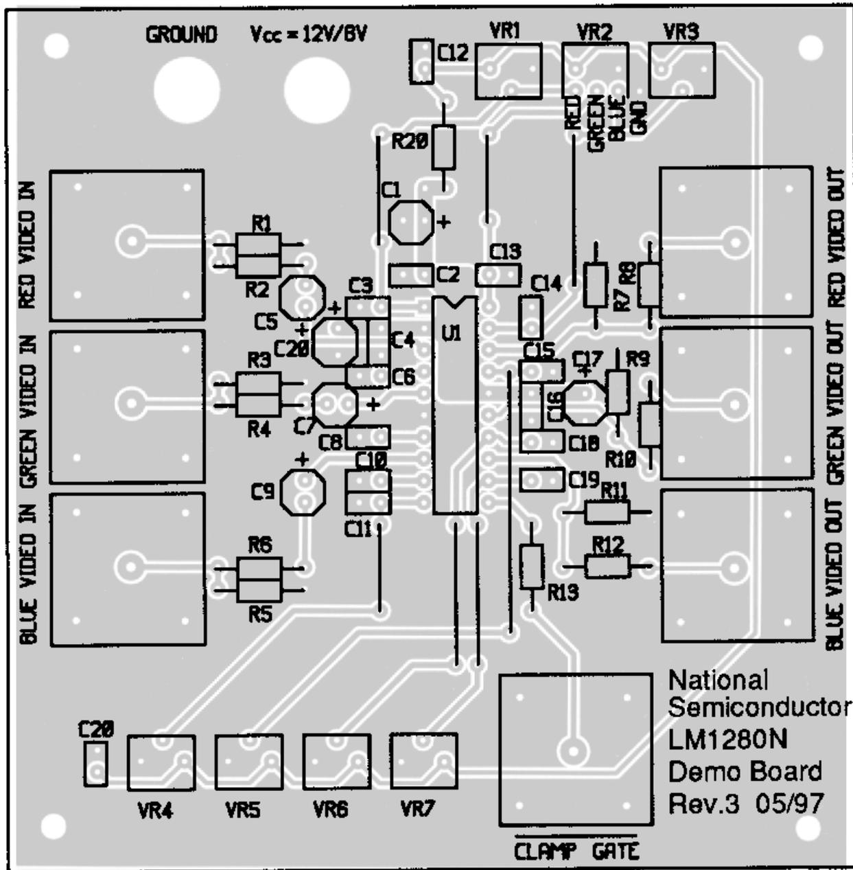
Figure 7. LM1279 OSD Video Pre-Amp Demonstration Board Layout
