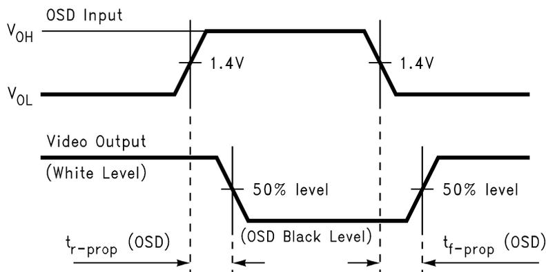
Figure 3. OSD Propagation Delays
