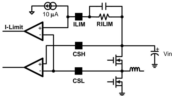
Figure 15. Current Sensing by Vds of the Top FET
