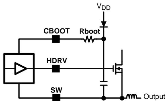
Figure 17. Adding a resistor in series with the CBOOT pin to suppress the turn-on switching noise
