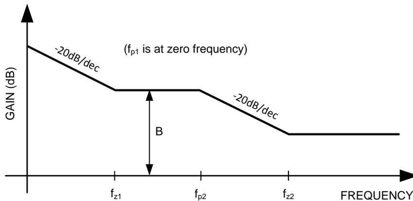
Figure 21. Output-Control Transfer Function
