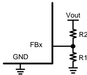
**Figure 18. Output Voltage Setting**
