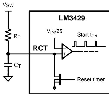
**Figure 15. Off-timer Circuitry for Boost and Buck-boost Regulators**
