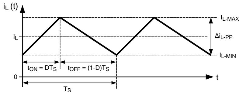
Figure 14. Ideal CCM Regulator Inductor Current  $i_L(t)$
