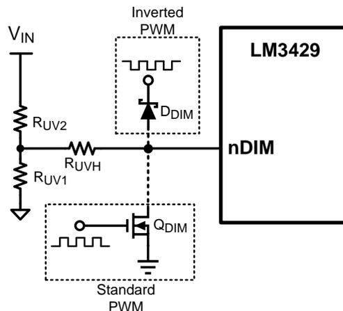
Figure 26. PWM Dimming Circuit
