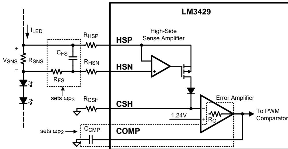
Figure 21. Compensation Circuitry
