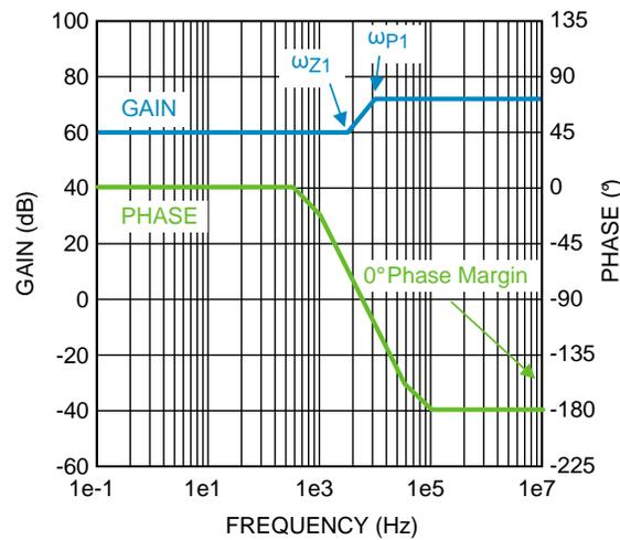
Figure 20. Uncompensated Loop Gain Frequency Response
