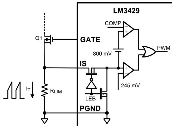
Figure 19. Current Sense / Current Limit Circuitry
