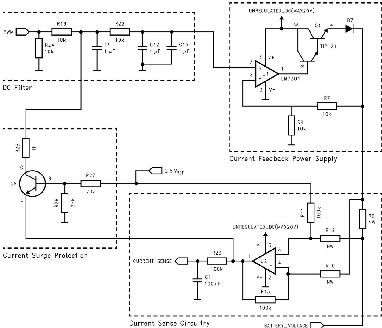
Figure 8. Circuitry Used for Li-Ion
