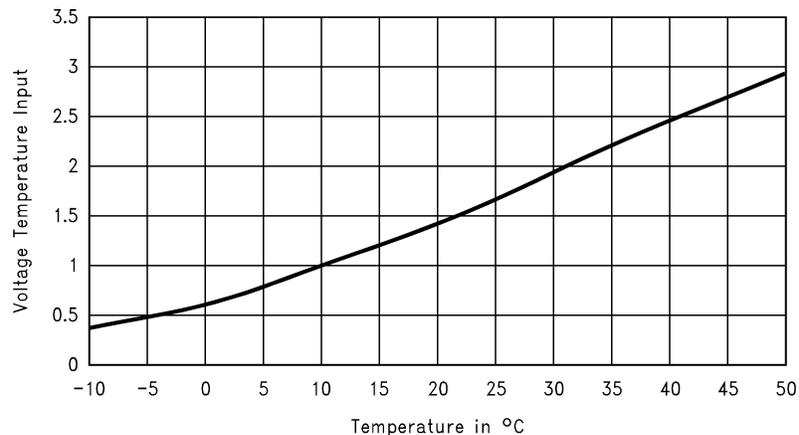
**Figure 5. Typical Configuration Curve, (NTC Characteristics:  $3\text{ k}\Omega$  @  $25^\circ\text{C}$ ,  $\beta=3988$ )**
