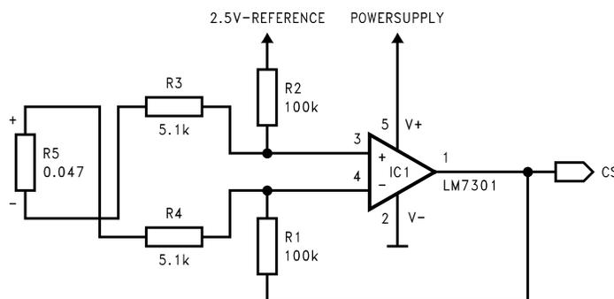
The current-sensing signal is amplified, inverted and centered on the 2.5V reference by the operational amplifier and fed into the CS pin on the LM3647. The amplification stage must be dimensioned by setting the appropriate ratio between R1 (R2) and R3 (R4). The figure above is dimensioned for a maximum current of about 1.1A. This was calculated using [Equation 4](#):
