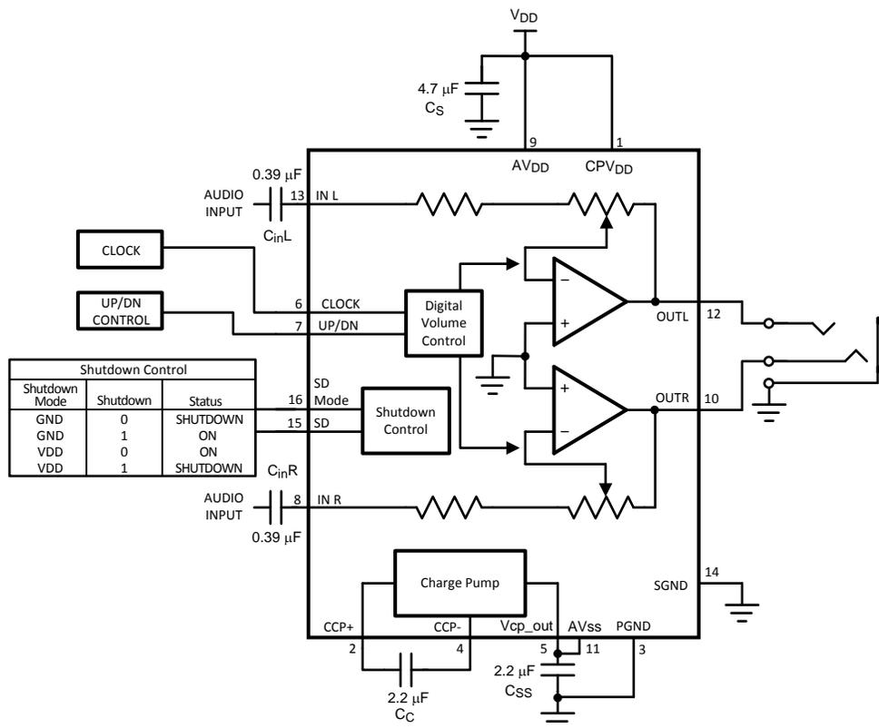
**Figure 2. Typical Audio Amplifier Application Circuit**
