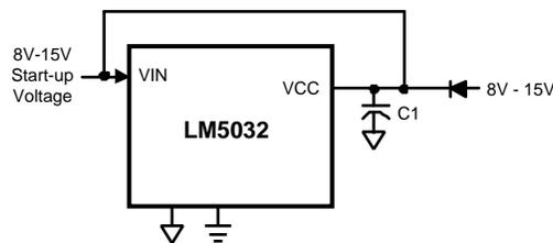
Figure 24. Bypassing the Internal Start-up Regulator
