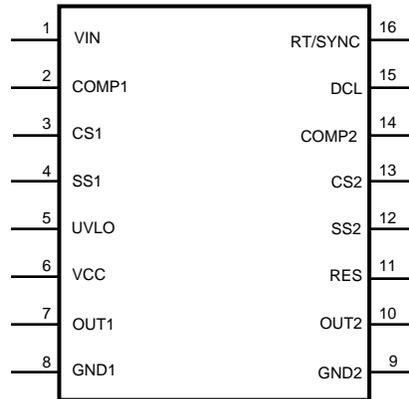
**Figure 2. 16-Lead TSSOP (Top View)
