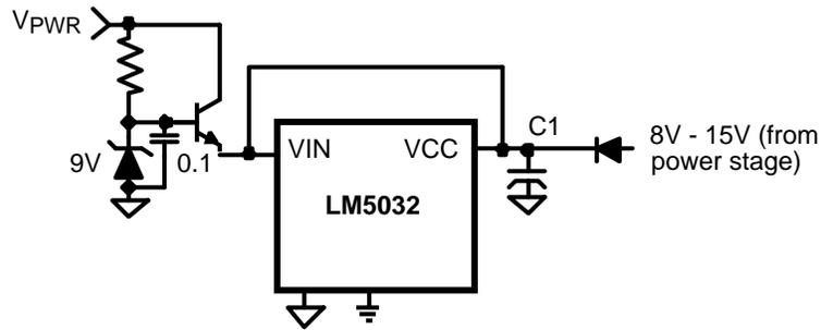
Figure 23. Start-up Regulator for  $V_{PWR} > 100V$
