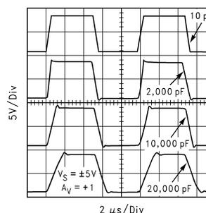
**Figure 2. Large Signal Step Response for Various Cap. Load**
