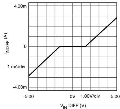
**Figure 38. Input Stage Current vs. Differential Input Voltage**
