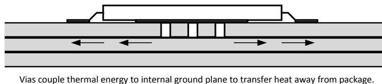
**Figure 5. 4 Layer PCB - Example 1**
