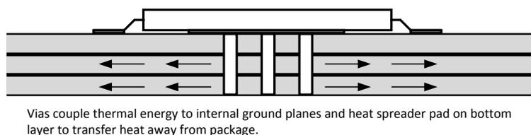
**Figure 6. 4 Layer PCB - Example 2**
