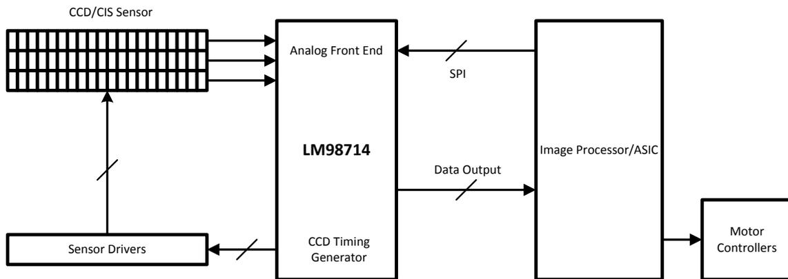
LM98714 Overall Chip Block Diagram
