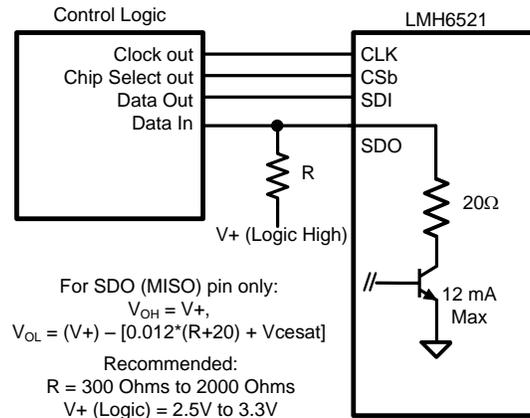
Figure 36. Serial Mode 4–wire Connection
