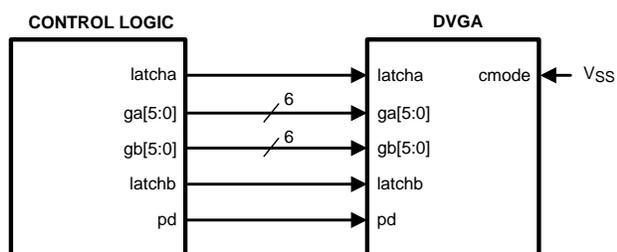
**Figure 32. Parallel Mode Connection for Fastest Response**
