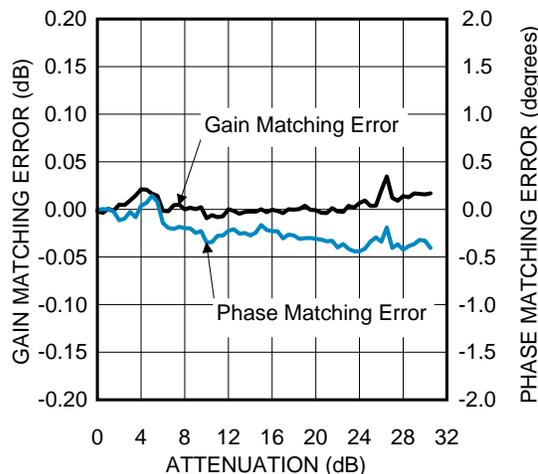
**Figure 2. Channel Matching Error (Ch A – Ch B)**
