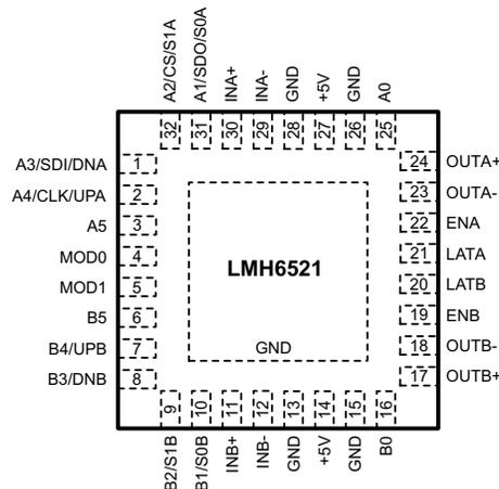
Figure 3. 32-Pin WQFN Package-Top View
