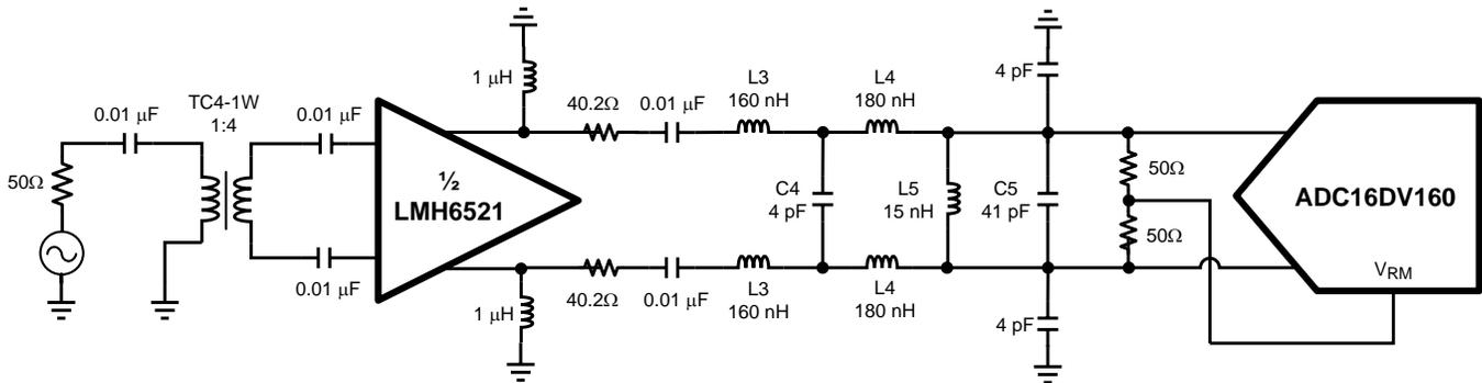
Center Frequency is 192MHz with a 20MHz Bandwidth. Designed for 200Ω Impedance.
