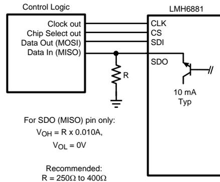
Figure 47. Internal Operation of the SDO pin
