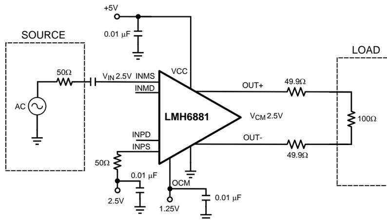
Figure 39. Typical Implementation with a Single-Ended Input Signal
