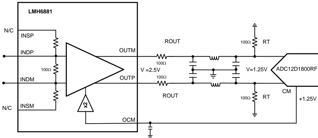
Figure 44. DC-Coupled ADC Driver Example 2, Terminated Input ADC
