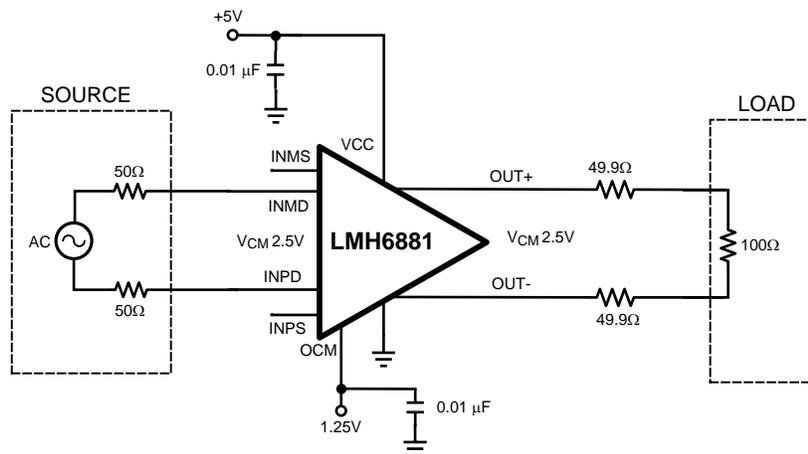
Figure 38. Typical Implementation with a Differential Input Signal
