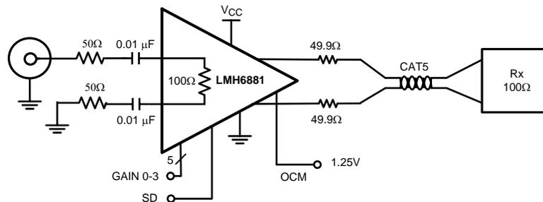
**Figure 37. LMH6881 Used as Twisted Pair Cable Driver**
