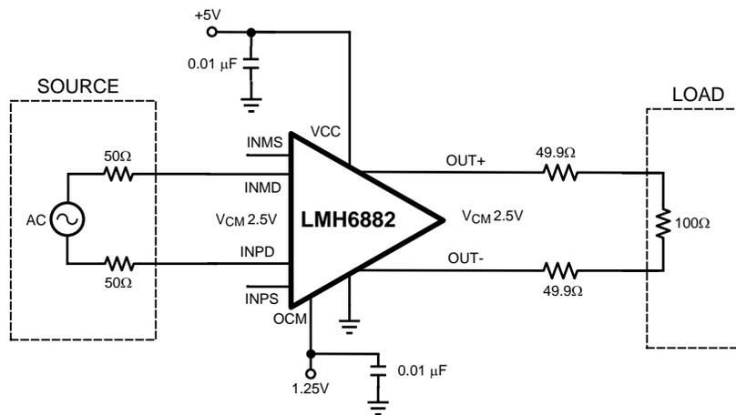
**Figure 42. Typical Implementation with a Differential Input Signal**
