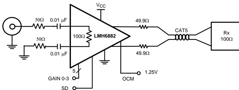
Figure 41. LMH6882 Used as Twisted Pair Cable Driver
