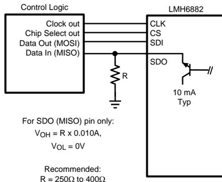
Figure 51. Internal Operation of the SDO Pin
