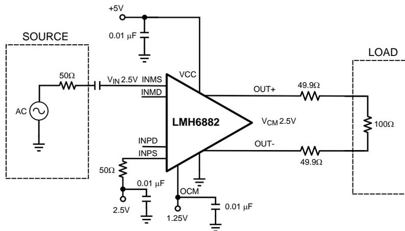
**Figure 43. Typical Implementation with a Single-Ended Input Signal**
