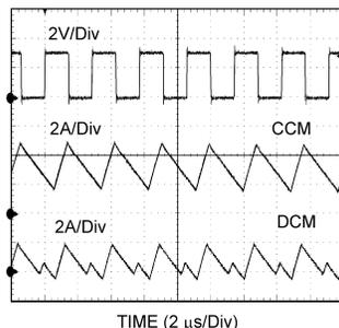
The approximate formula for determining the DCM/CCM boundary is as follows:
