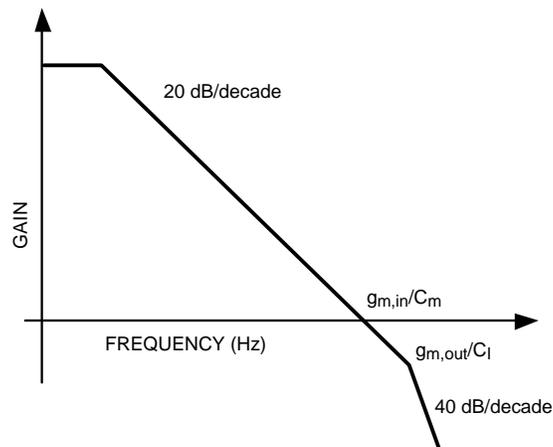
Figure 40. Bode Plot of the Frequency Response
