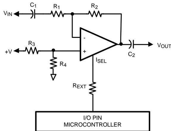
Figure 39. Inverting AC Coupled Application
