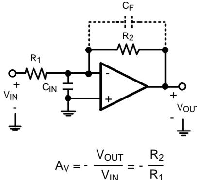
**Figure 43. Inverting Amplifier**
