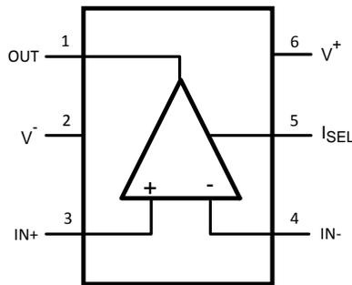
**Figure 2. 6-Pin SOT – Top View**
