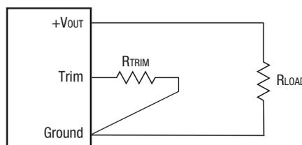
$$R_{TRIM} (k\Omega) = \frac{1.182}{V_{OUT} - 0.591}$$
