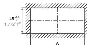
When n timers are continuously installed, the dimension (A) is calculated according to the following formula (n: the number of the timers to be installed):
