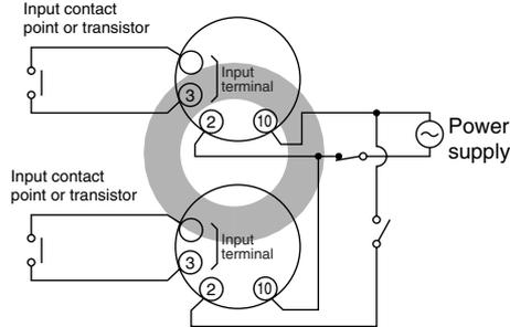
When power circuitry is not independent, one input signal can be fed to two or more counters at once, as shown in Fig. C.
