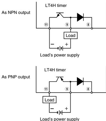
Note: With the 8-pin type, there is no diode between points ⑧ and ⑨.
