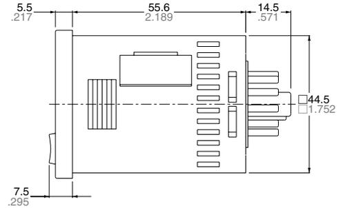
• Dimensions for embedded installation (with adapter installed)
