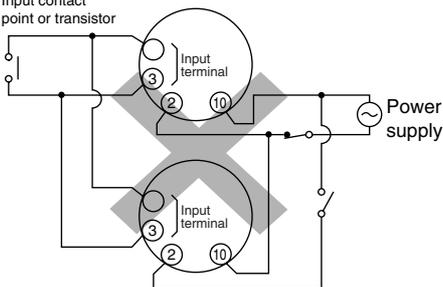
If independent power circuitry must be used, keep the input contacts or transistors separate from each other, as shown in Fig. B.
