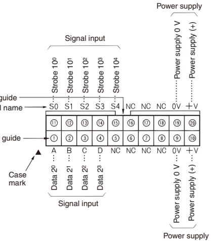
**Note:** Circled numbers are for the user's convenience. When preparing a socket, pay attention when wiring the terminals to the direction of the polarity guide.
