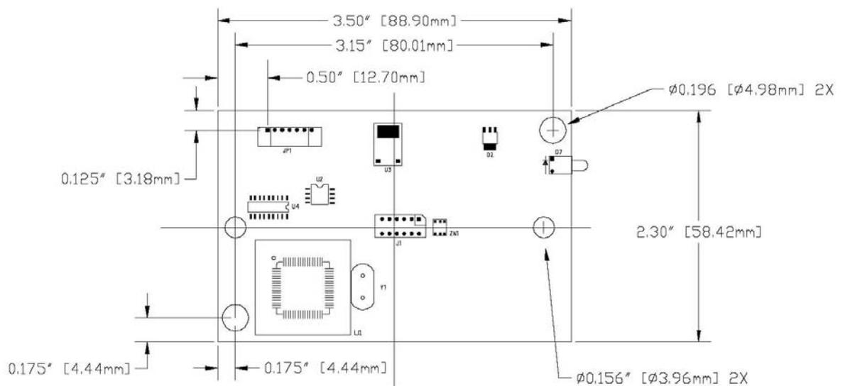
**Figure 2 Cased EX122 Touch Controller**
