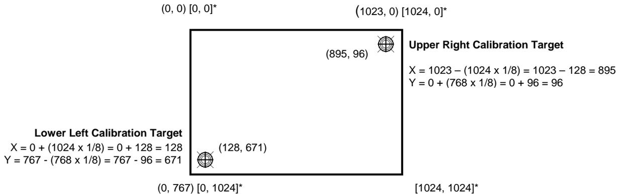
\*The coordinates are in *video* terms, with the origin (0, 0) in the upper left corner of the sensor. Examples from the *controller's* perspective, however, place the origin at the lower left corner of the sensor (numbers in brackets). The controller outputs 0 to 64K on both axes independent of display screen resolution.
