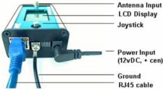
The 3M EM Aware TNG ESD Event Monitor is controlled using a 5-way joystick on the right side of the screen; 1) Left, 2) Right 3) Up, 4) Down, and 5) Push. They will be referred as L, R, U, D and P in this guide.
