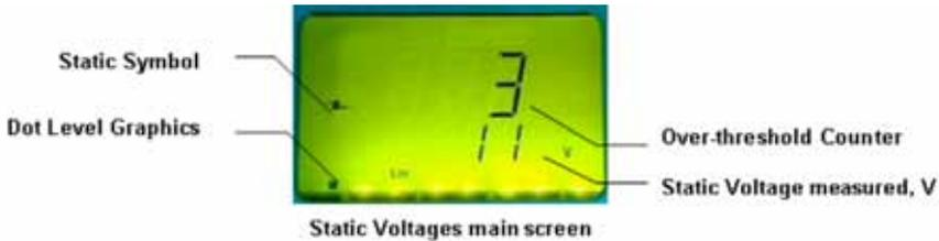
1. At the main screen display (no “REF” symbol), move the joystick until the display is as shown above.
