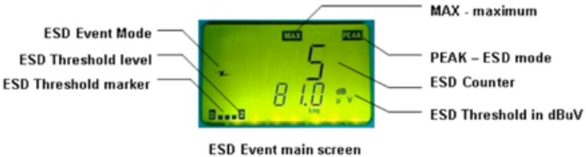
1. To reset the ESD counter to zero, press the joystick momentarily.
