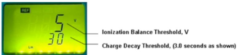
6. Move the joystick up or down to increase or decrease the decay time threshold.
