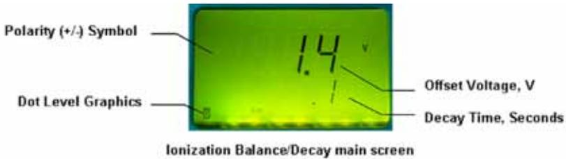
1. At the main screen display (no “REF” symbol), move the joystick until the display is as shown similar above.
