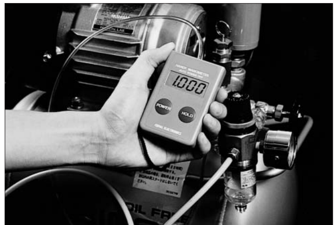
▲ Measurement of source pressure from a compressor.
