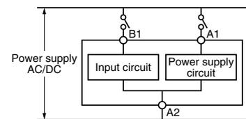
• Since input circuit and power supply circuit is independent, it is possible to switch ON and OFF for input circuit regardless power ON and OFF. Note that the contact of input circuit is given same voltage as power voltage.
