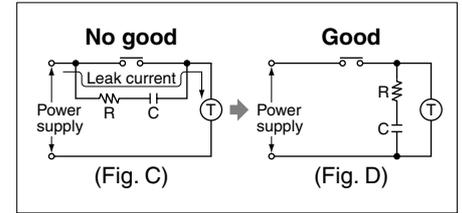
4. In order to maintain the characteristics of the timer, long continuous current flow through the timer, causing generation of heat internally should be avoided because of the degradation it can cause. For such long continuous operation, the circuit shown below should be used.
