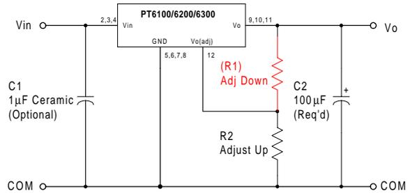
The values of (R1) [adjust down], and R2 [adjust up], can also be calculated using the following formulae.
