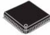
PLQP0112JA-A 20×20mm, 0.65mm pitch PLQP0100KB-A 14×14mm, 0.5mm pitch PLQP0080JA-A 14×14mm, 0.65mm pitch PLQP0064KB-A 10×10mm, 0.5mm pitch PLQP0064GA-A 14×14 mm, 0.8mm pitch
