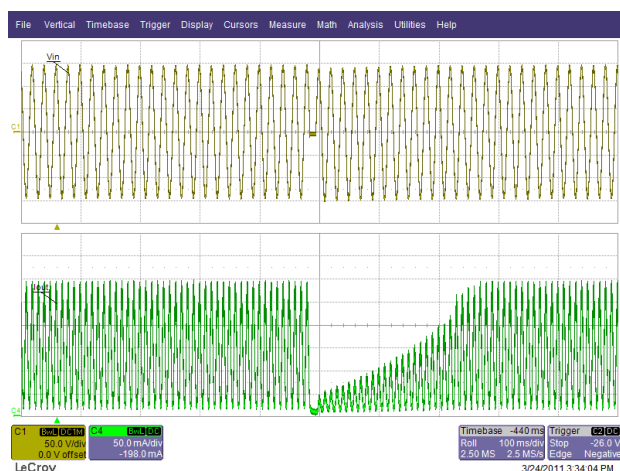
Figure 43 – 115 VAC / 50 Hz, 0.5 Cycle-Skip. Load: 35 V LED String. Ch1: V_{IN} , 50 V / div. Ch3: I_{IN} , 50 mA / div, 100 ms / div.
