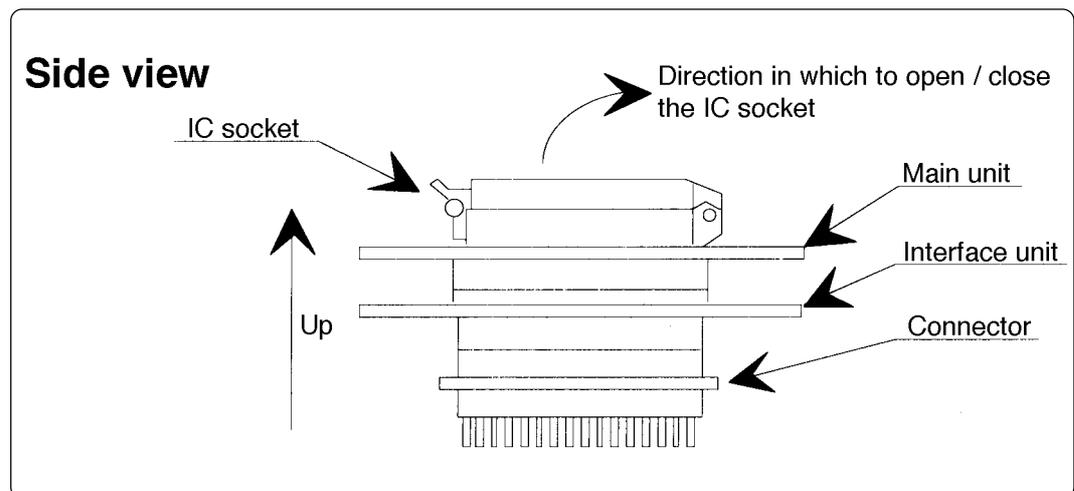
Figure 4.4 Opening and closing the IC socket
