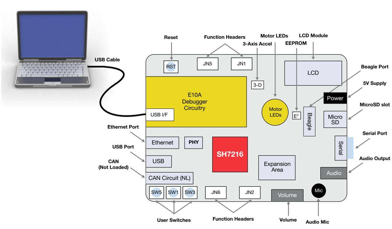
Figure 5-2: RDK Connections
