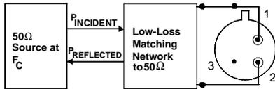
$$\text{CW RF Power Dissipation} = P_{\text{INCIDENT}} - P_{\text{REFLECTED}}$$
