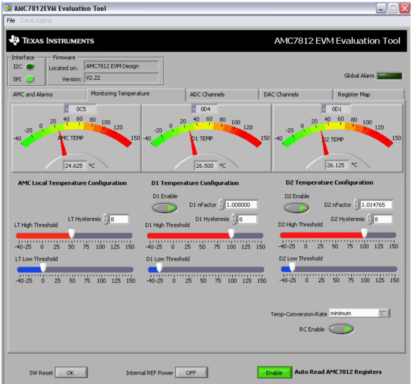
**Figure 4. AMC7812EVM-PDK Software GUI: Start-Up Screen with Monitoring Temp Tab**
