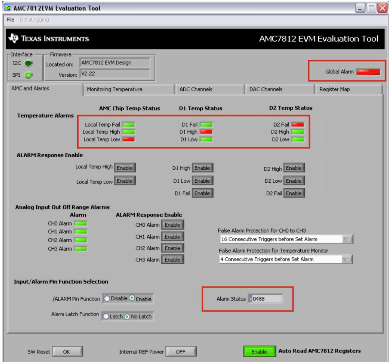
Figure 7. AMC7812EVM-PDK Software GUI: Alarms Triggered
