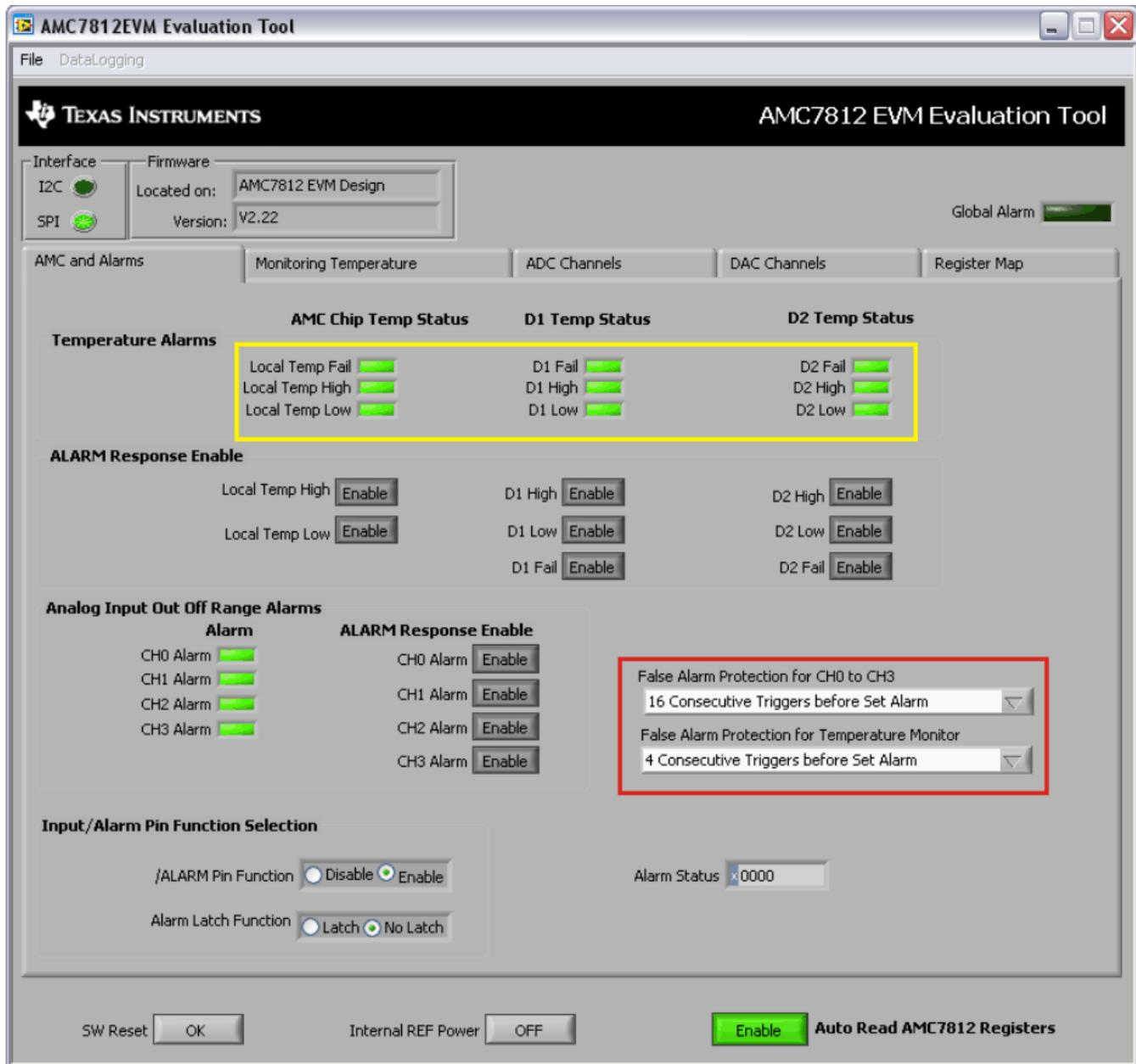
Figure 6. AMC7812EVM-PDK Software GUI: AMC and Alarms Tab
