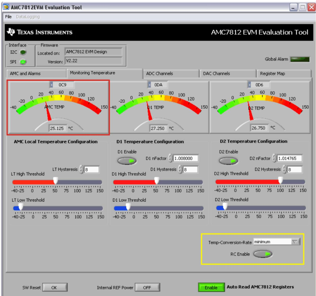
Figure 8. AMC7812EVM-PDK Software GUI: Monitoring Temperature Tab
