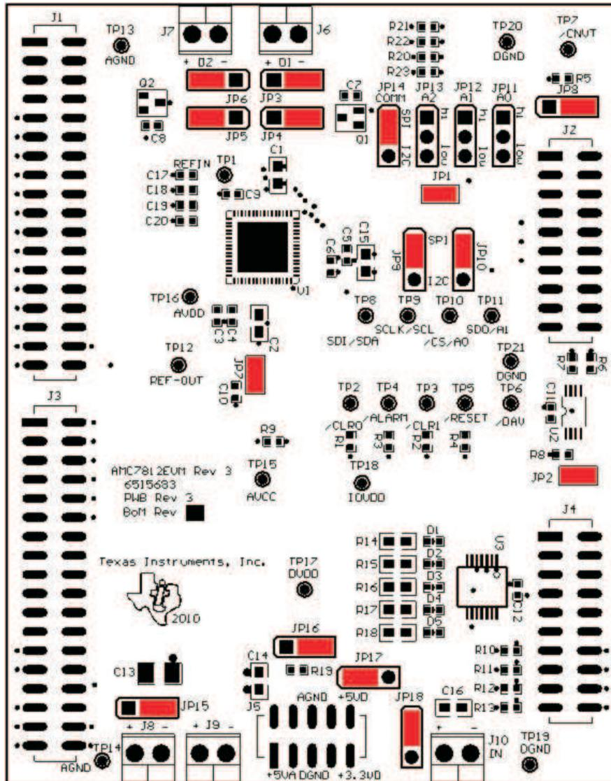
Figure 1. Default Jumper Configuration
