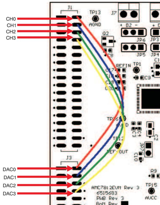
**Figure 12. Connections on AMC7812EVM Board for Running Analog Loopback Test**
