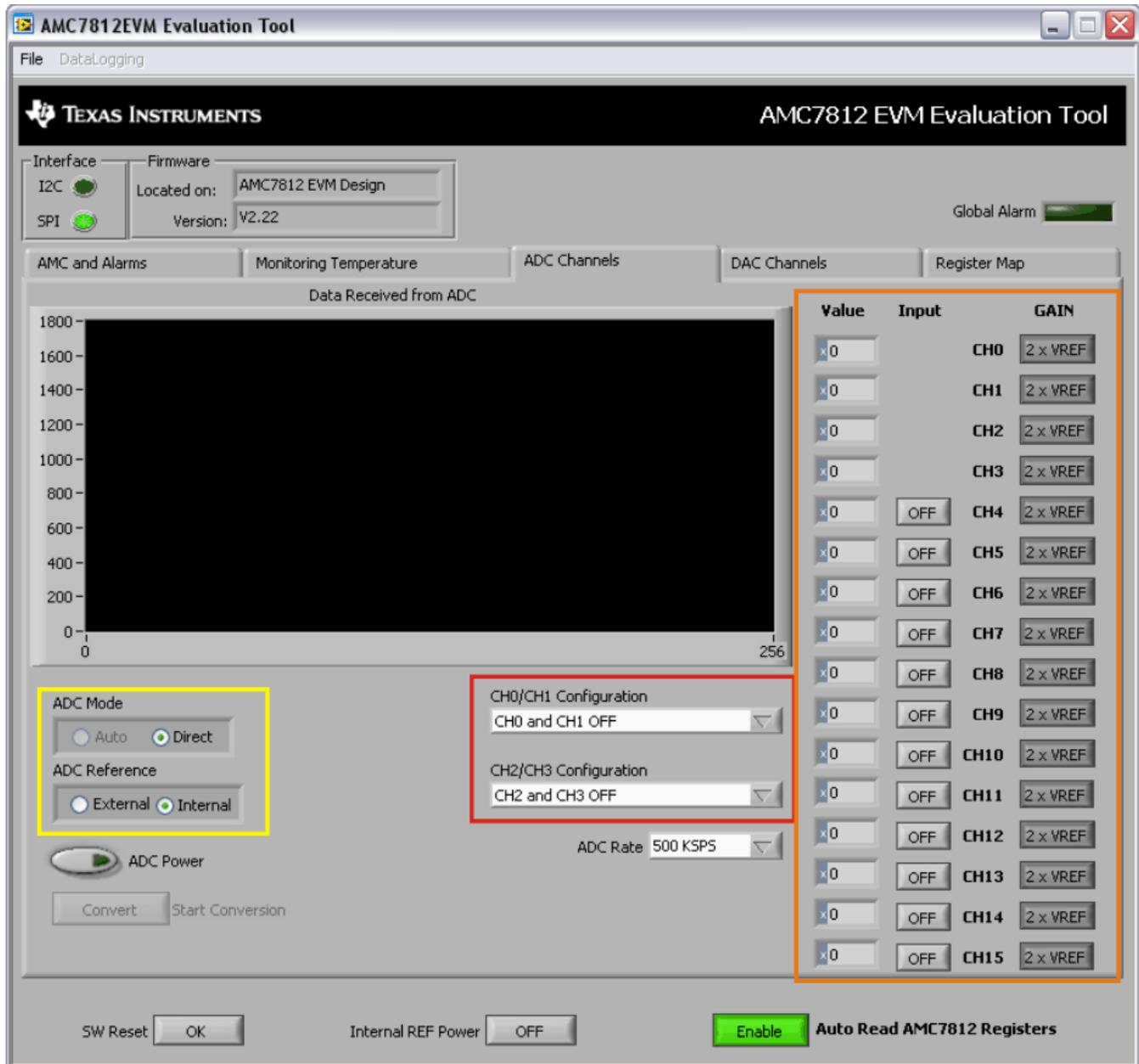
Figure 9. AMC7812EVM-PDK Software GUI: ADC Channels Tab
