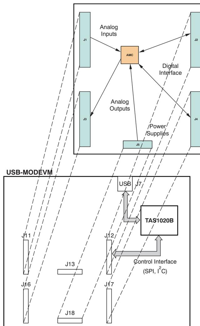
**Figure 2. AMC7812EVM-PDK Hardware Block Diagram and Connections**
