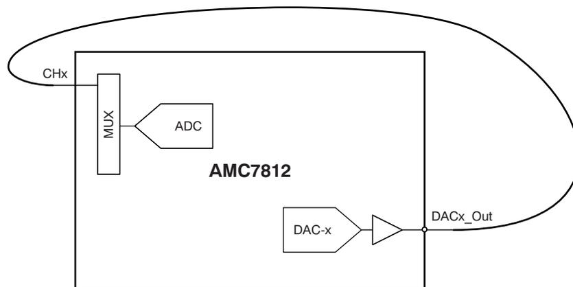
**Figure 11. AMC7812 Analog Loopback Test**
