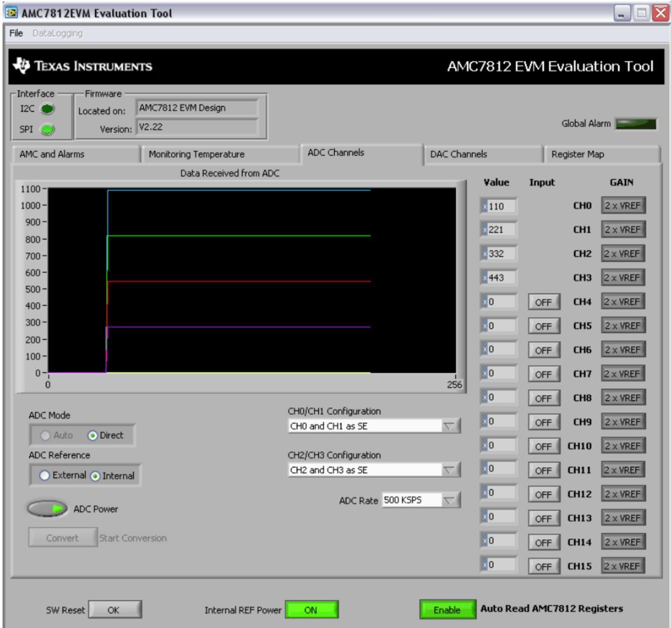
**Figure 13. AMC7812EVM-PDK Software GUI: Analog Loopback Test of CH0–CH3**
