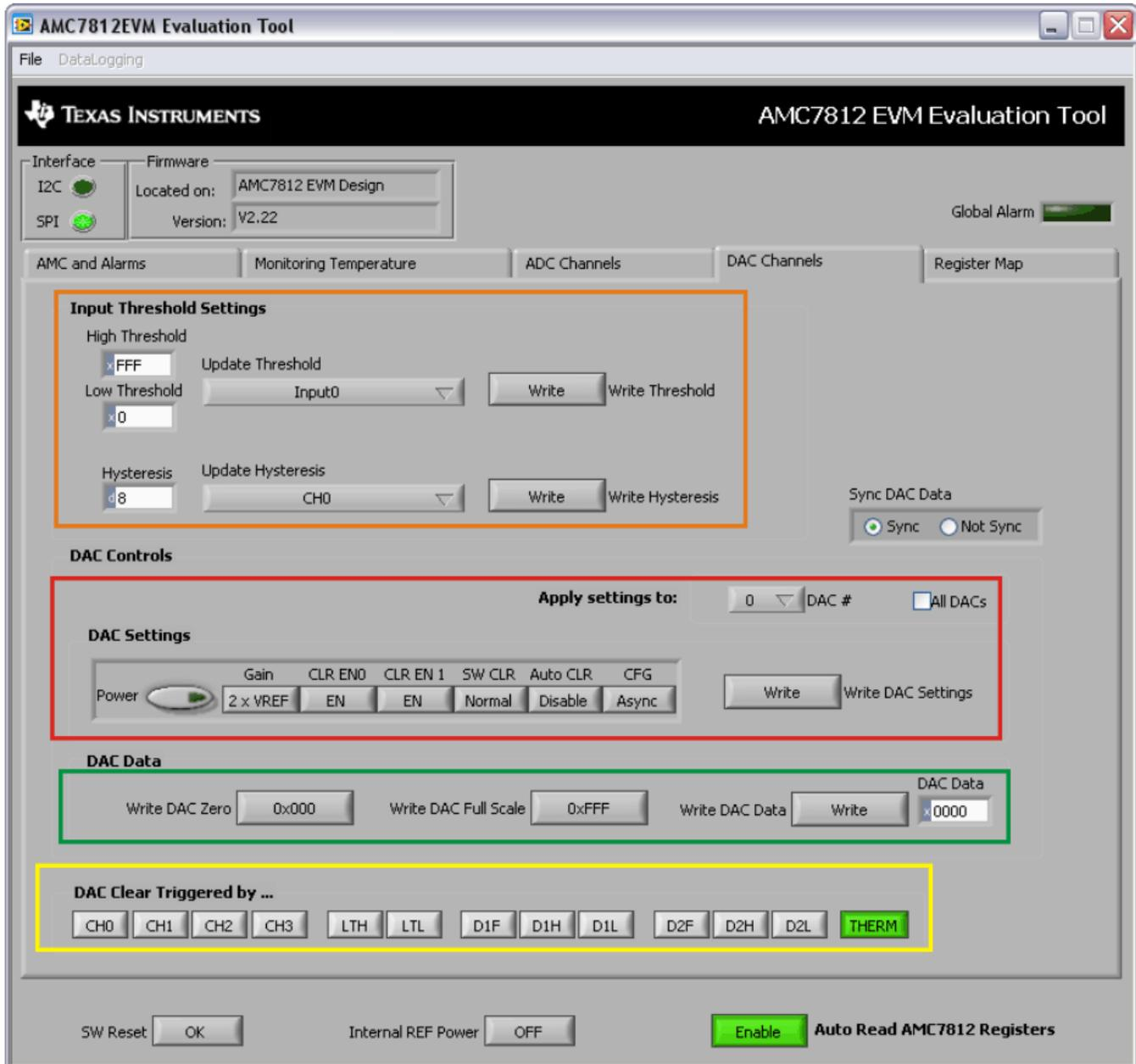
Figure 10. AMC7812EVM-PDK Software GUI: DAC Channels Tab
