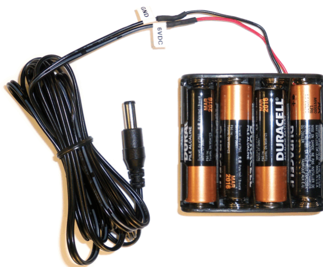
Figure 53. Recommended Power Supply for ADS1298R
