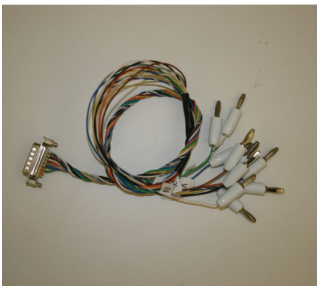
Figure 50. 15-Pin, Twisted Wire Cable to Banana Jacks
