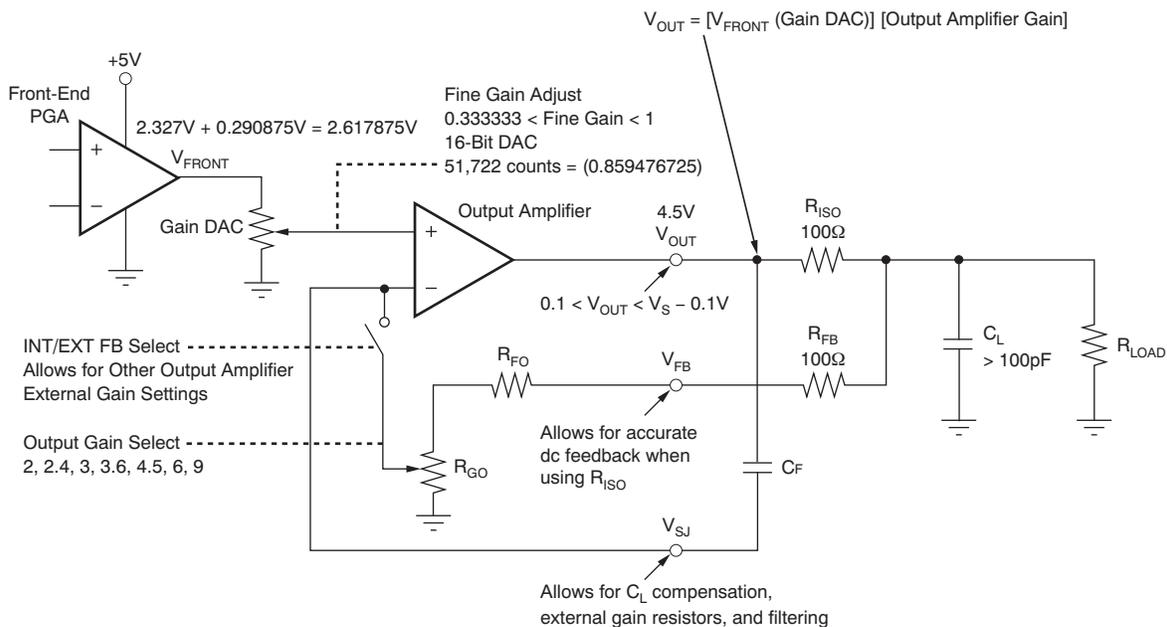
NOTE:  $V_{OUT} = [(V_{DIFF} + V_{COARSE\ OFFSET})(Front\text{-}End\ PGA\ Gain) + V_{ZERO\ DAC}][Gain\ DAC][Output\ Amplifier\ Gain]$
