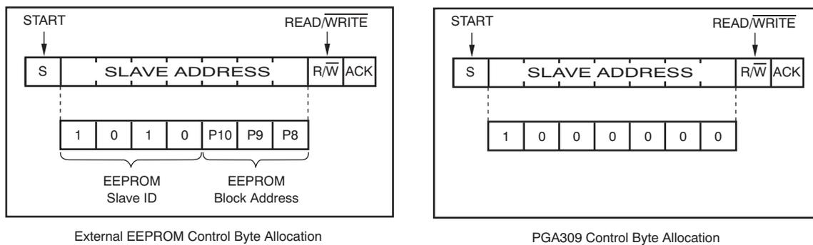
Figure 4-3. External EEPROM and Control Byte Allocation
