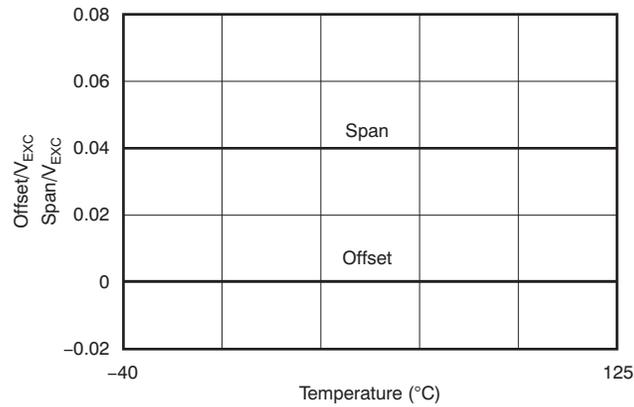
Figure 5-3. Ideal Span and Offset vs Temperature
