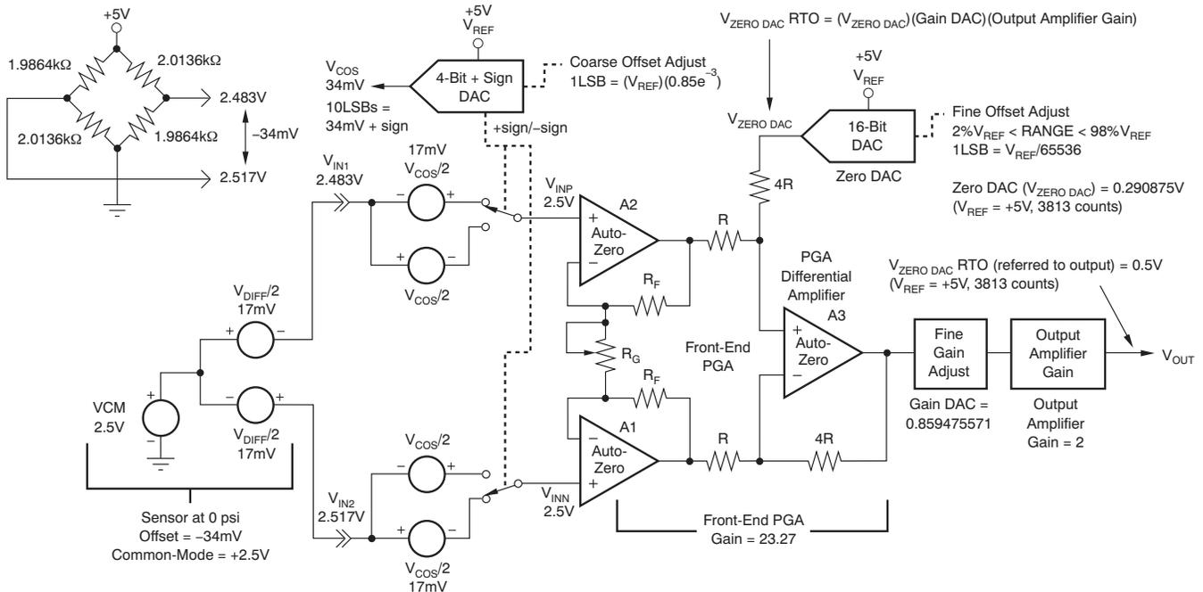
NOTE:  $V_{OUT} = [(V_{DIFF} + V_{COARSE OFFSET})(\text{Front-End PGA Gain}) + V_{ZERO DAC}][\text{Gain DAC}][\text{Output Amplifier Gain}]$
