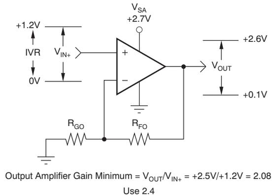
**Figure 2-7. Output Amplifier Minimum Gain at Low Supply**
