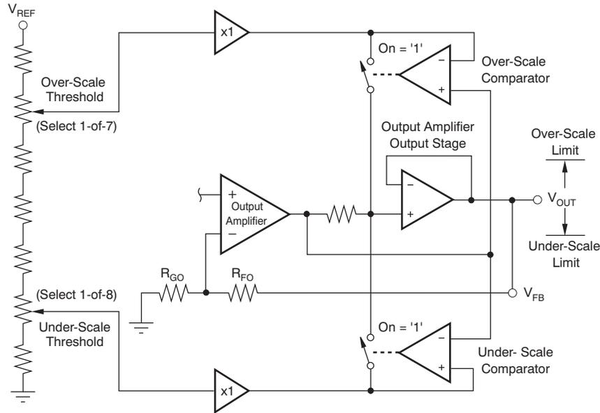
Figure 2-24. Over-Scale and Under-Scale Limit Circuit
