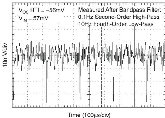
Figure 2-37. 0.1Hz to 10Hz  $V_{OUT}$  Peak-to-Peak Noise for Coarse Offset Adjust =  $-56\text{mV}$ , Gain = 1152,  $V_{IN} = +57\text{mV}$ , CLK\_CFG = '11',  $V_{NPP}$  (RTI) =  $42\mu\text{V}_{PP}$
