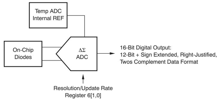
**Figure 6-3. Internal Temperature Mode (Register 6 [9] = '1')**
