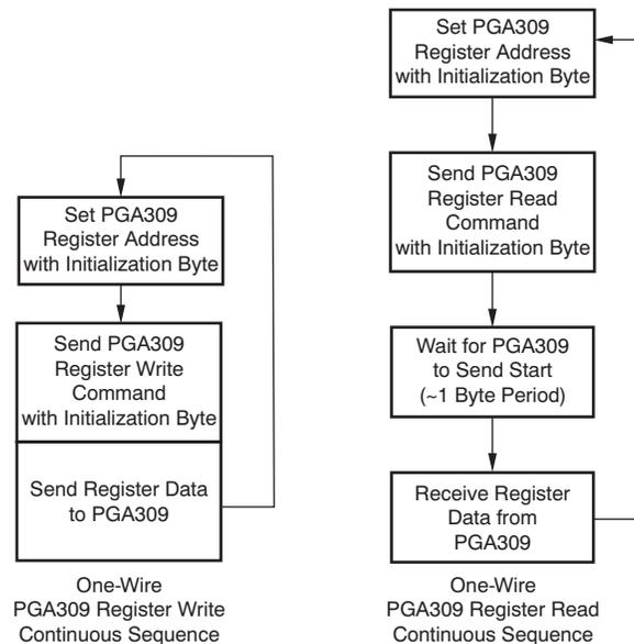
Figure 4-7. One-Wire Access to PGA309 Registers
