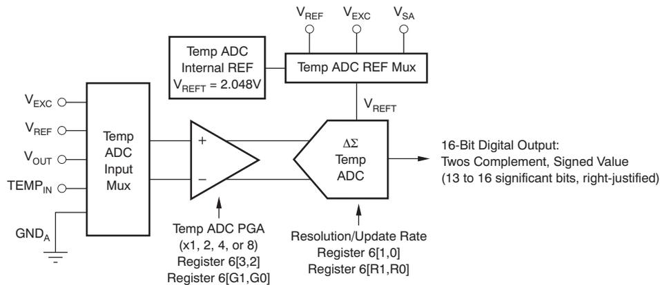
**Figure 6-4. External Signal Mode (Register 6 [9], TEN = '0')**
