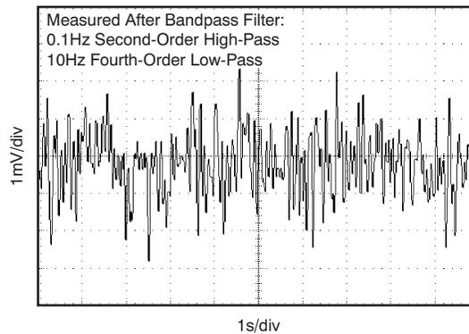
**Figure 2-33. 0.1Hz to 10Hz  $V_{OUT}$  Peak-to-Peak Noise for Coarse Offset Adjust = -56mV, Gain = 1152,  $V_{IN}$  = +57mV, CLK\_CFG = '01',  $V_{NPP}$  (RTI) = 4.44  $V_{PP}$**
