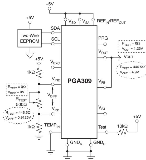
NOTE: Two conditions for  $V_{DIFF}$  and the resulting  $V_{OUT}$  are shown in this figure. Condition one is in a dashed, square box. Condition two is shown in a dashed oval.
