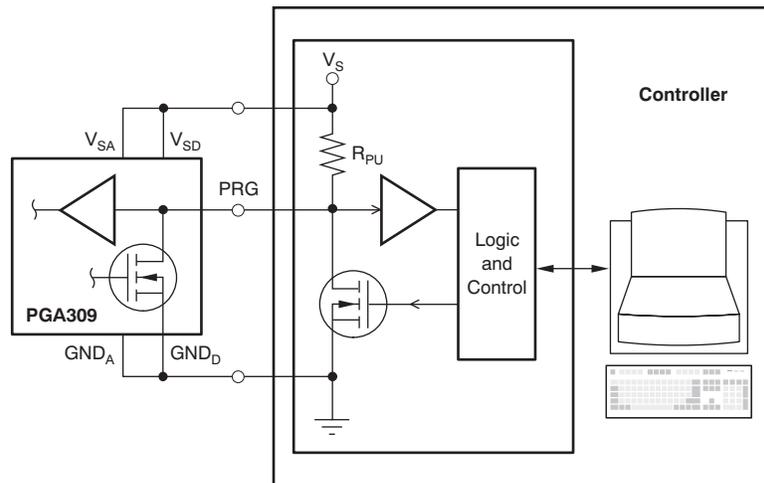
Figure 4-5. Typical PGA309 PRG To Controller Connection
