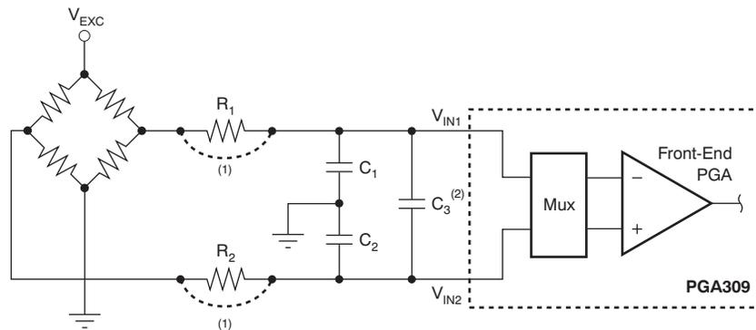
**Figure 2-39. Input Filtering**
