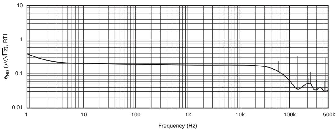
**Figure 2-34.  $V_{OUT}$  Noise Spectrum for Coarse Offset Adjust = -56mV, Gain = 1152,  $V_{IN}$  = +57mV, CLK\_CFG = '01'**
