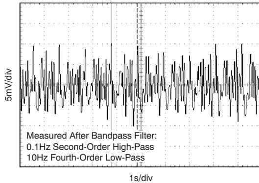
Figure 2-35. 0.1Hz to 10Hz  $V_{OUT}$  Peak-to-Peak Noise for Coarse Offset Adjust =  $-56\text{mV}$ , Gain = 1152,  $V_{IN} = +57\text{mV}$ , CLK\_CFG = '10',  $V_{NPP}$  (RTI) =  $18.4\mu\text{V}_{PP}$
