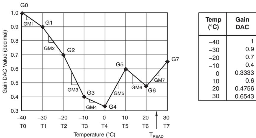
Figure 3-3. Desired Gain DAC Values
