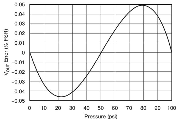
**Figure 2-14. Corrected Bridge Parabolic Nonlinearity vs Pressure**
