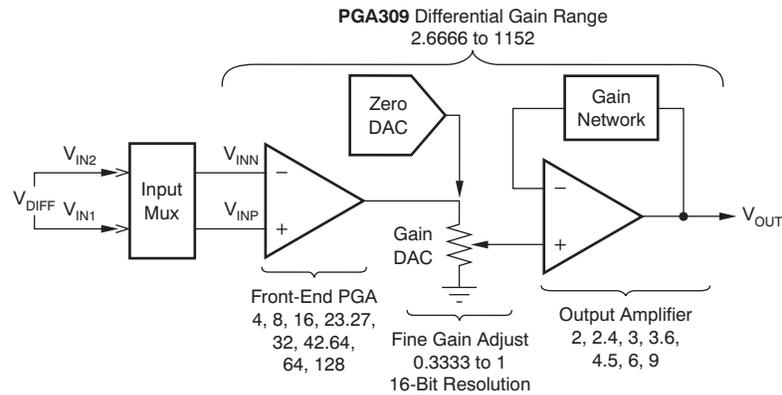
$$\text{NOTE: } V_{\text{OUT}} = [(V_{\text{DIFF}} + V_{\text{COARSE OFFSET}})(\text{Front-End PGA Gain}) + V_{\text{ZERO DAC}}][\text{Gain DAC}][\text{Output Amplifier Gain}]$$
