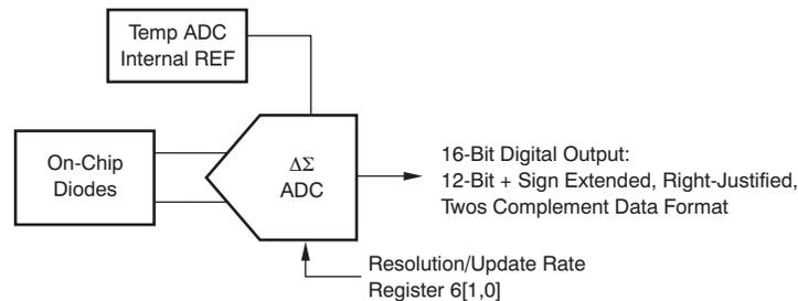
**Figure 6-1. Internal Temperature Mode; Register 6[9] = '1'**
