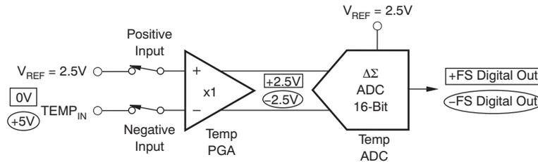
**Figure 6-2. External Signal Mode; Register 6 = '0000 0100 0011 0000'**
