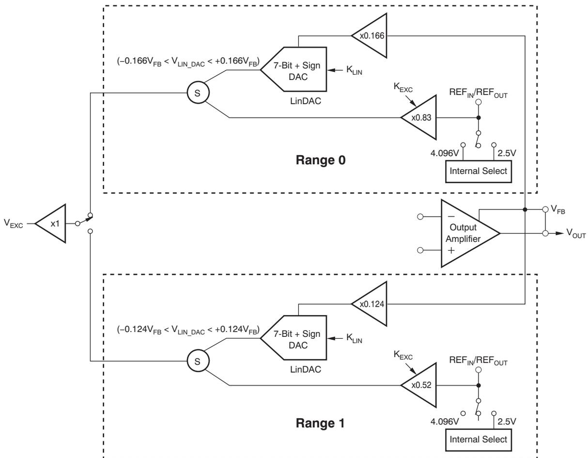
Figure 2-11. Linearization Circuit
