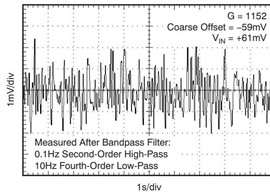
**Figure 2-28.  $V_{OUT}$  Noise, 0.1Hz to 10Hz Peak-to-Peak Noise**
