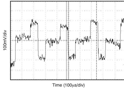
Figure 2-30. Unfiltered  $V_{OUT}$  Clock Feedthrough Glitch, Coarse Offset Adjust =  $-59\text{mV}$ , Gain = 1152,  $V_{IN} = +61\text{mV}$ , CLK\_CFG = '00' (default).  $V_{OUT}$  Glitch (RTI) =  $347\mu\text{V}_{PP}$
