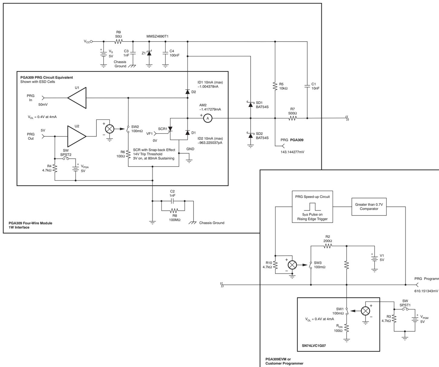
Figure 4-20. PRG Circuit Protection Logic Levels
