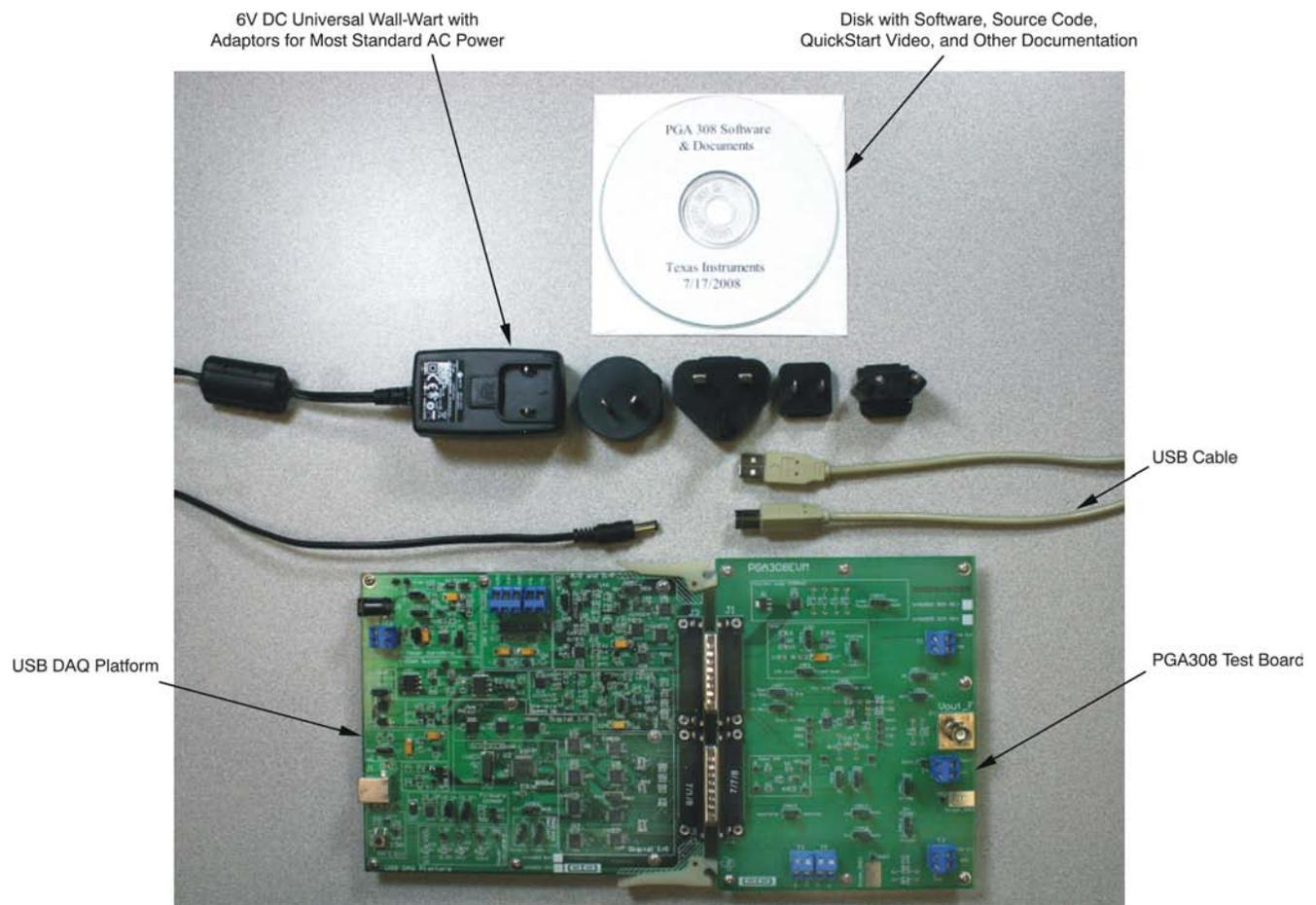
**Figure 1-1. Hardware Included with the PGA308EVM**
