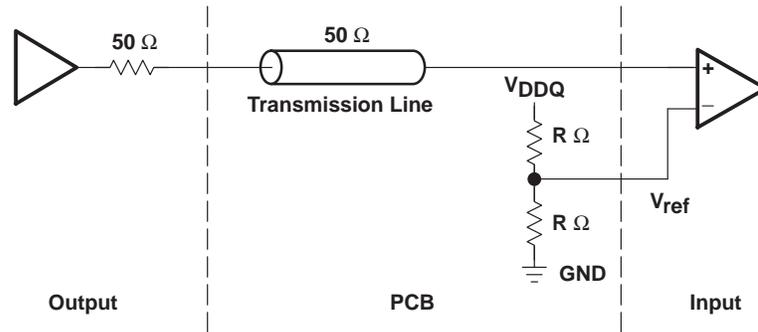
NOTE: The TLK3104SA provides a push-pull effect on the output buffer for externally sourced series terminated loads. In HSTL mode, the signal swing is very small, allowing for minimal power consumption and low electromagnetic emission (EME). To assure sufficient signal levels on the receive side, no termination resistor is used.
