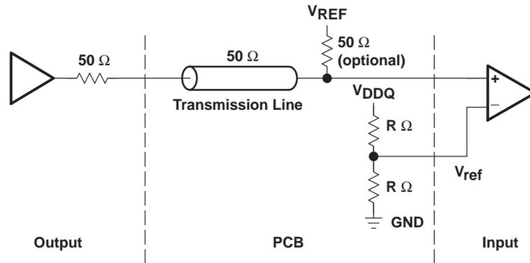
NOTE: The output buffer of the TLK3104SA has on-chip termination of 50 Ω. The output signal is compliant with the JEDEC SSTL\_2 Class 1 specification. Line termination on the receive end is optional and not recommended for low-power applications.
