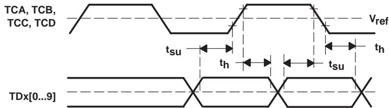
**Figure 22. SSTL\_2 CLASS1/1.8V HSTL Input Timing Requirements**
