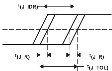
NOTE:  $t(J\_TOL) = t(J\_R) + t(J\_IDR)$ , where  $t(J\_TOL)$  is the receive jitter tolerance,  $t(J\_IDR)$  is the received deterministic jitter, and  $t(J\_R)$  is the Gaussian random edge jitter distribution at a maximum BER =  $10^{-12}$ .
