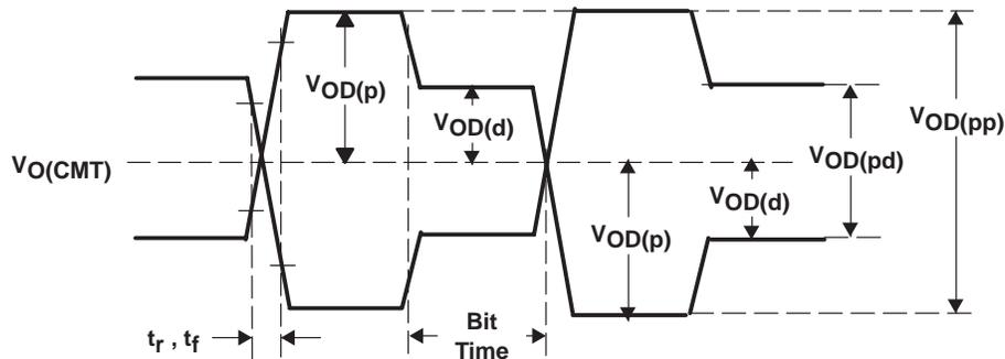
**Figure 17. Differential and Common-Mode Output Voltage Definitions**
