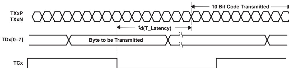
Figure 5. Transmitter Latency
