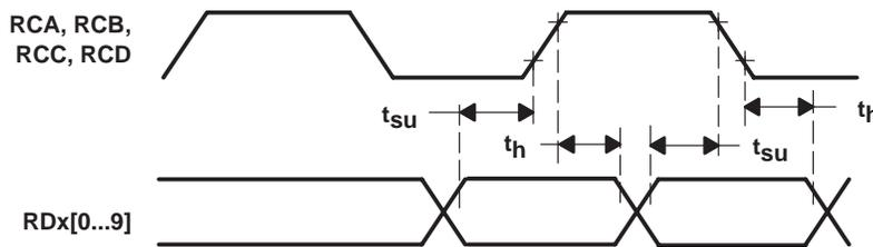
Figure 21. SSTL\_2 CLASS1/1.8V HSTL Output Timing Requirements
