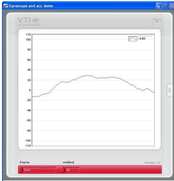
**Gyro**, continuously scrolling gyro output. Angular rate is presented in [ $^{\circ}$ /s].
