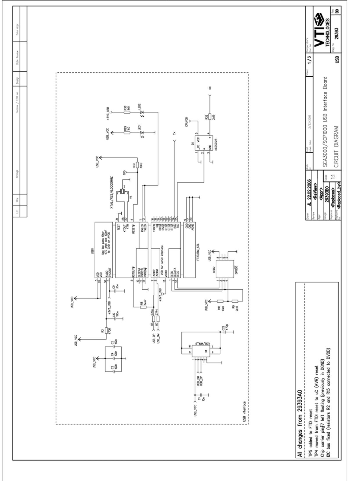
Figure 11. SCC1300 Demo Kit USB interface board circuit diagram (sheet USB).
