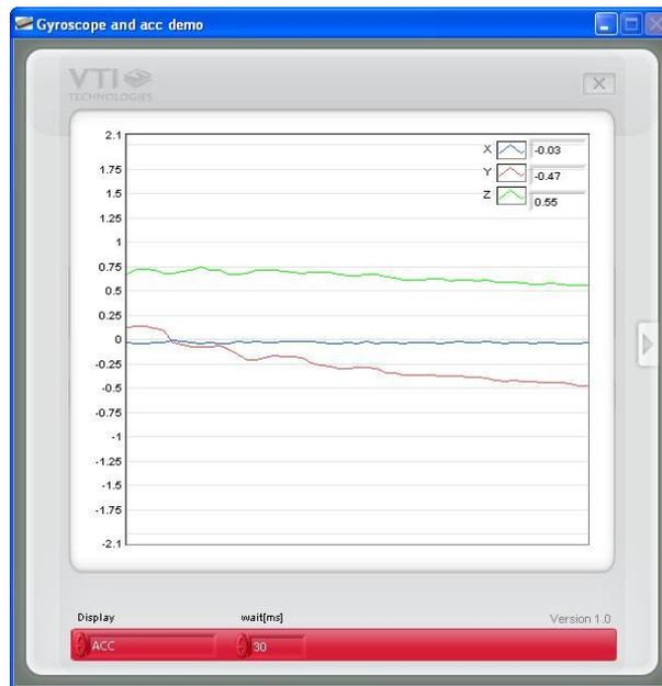
**ACC**, continuously scrolling X, Y and Z outputs of the accelerometer. Acceleration is presented in [g].
