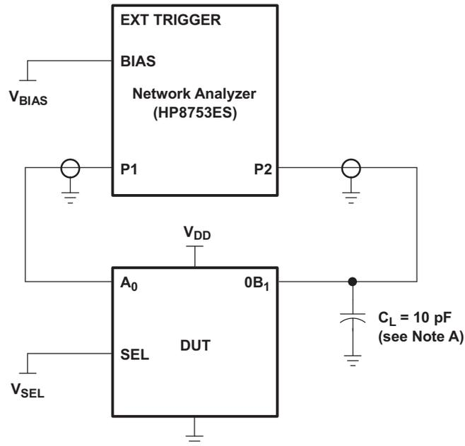
A. C<sub>L</sub> includes probe and jig capacitance.
