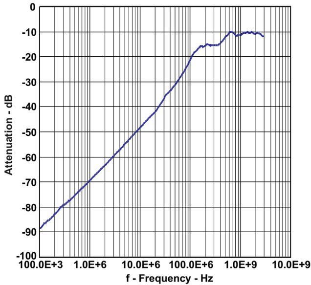
Figure 5. Off Isolation vs Frequency for Audio Switch
