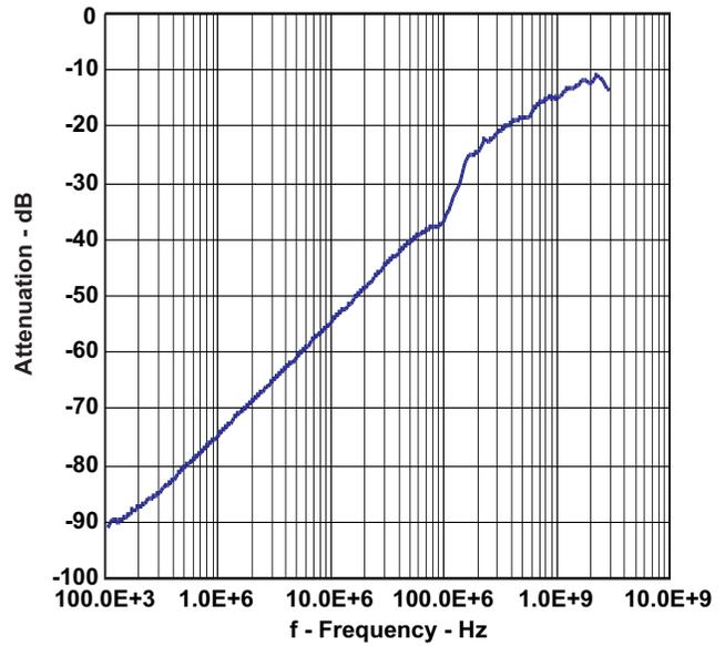
Figure 6. Off Isolation vs Frequency for USB Switch
