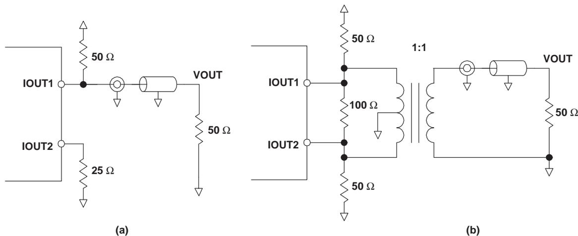
**Figure 28. Driving a Doubly Terminated 50 Ω Cable**
