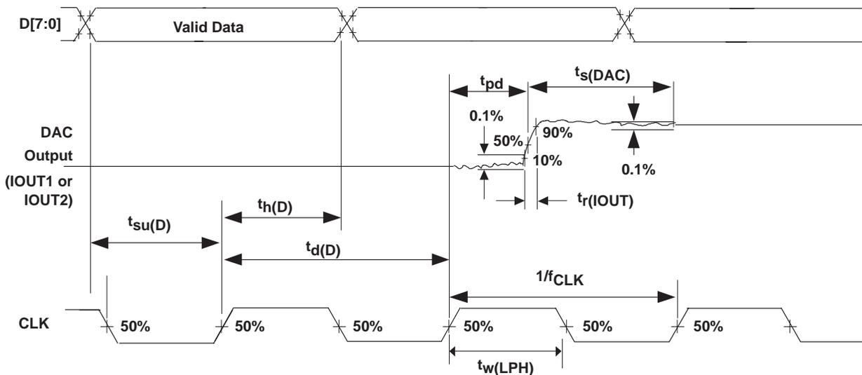
Figure 23. Timing Diagram
