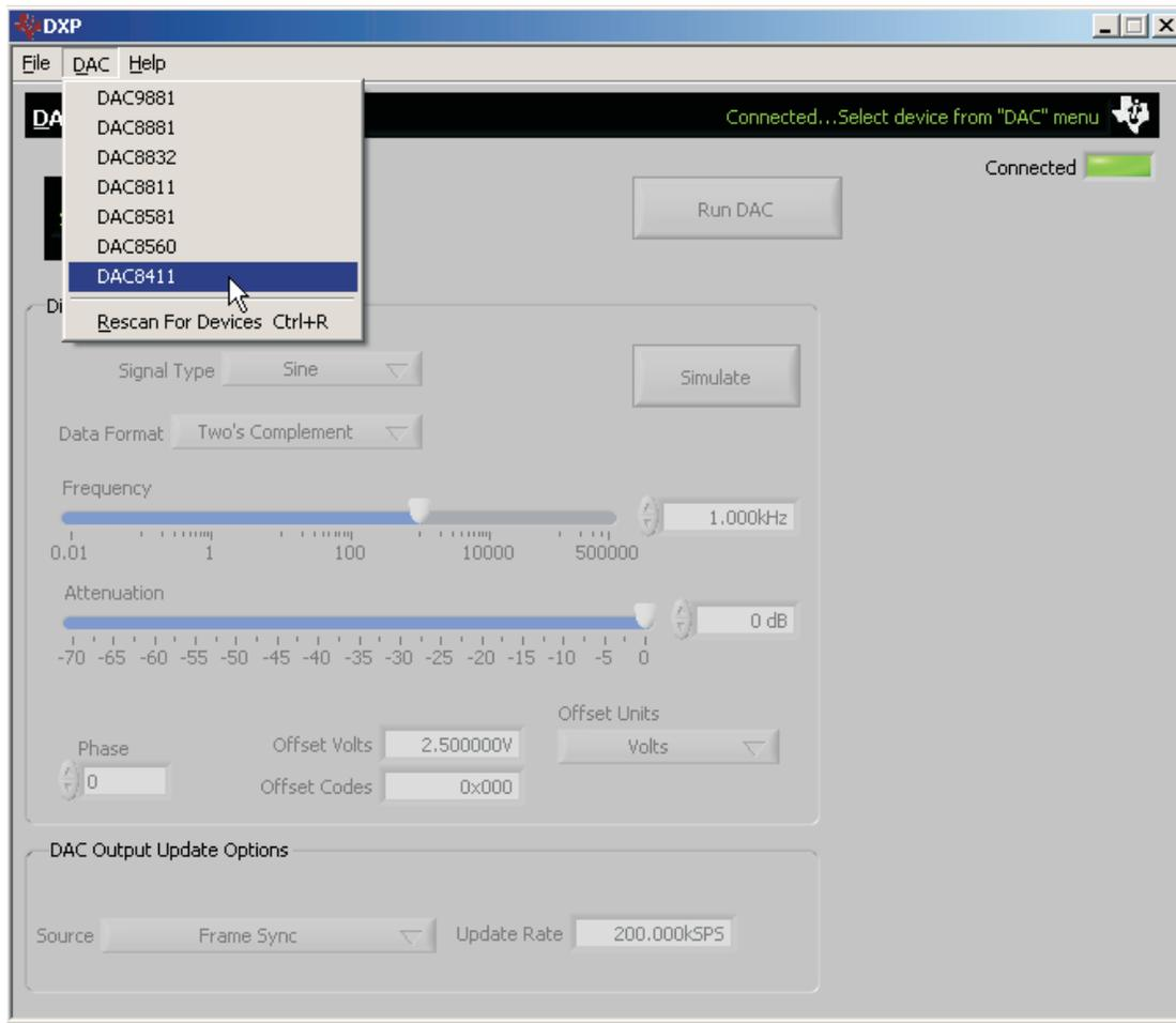
**Figure 2. Loading a SC70 DAC EVM Configuration**
