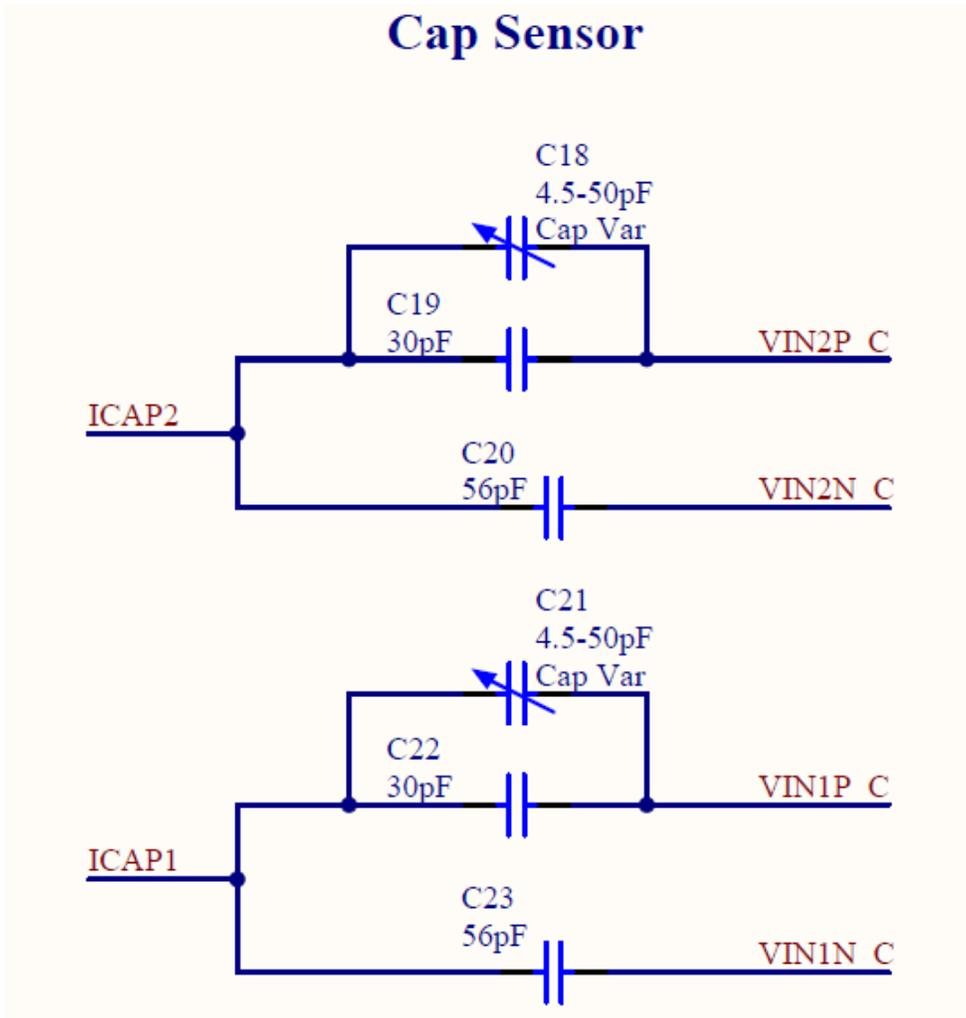
Figure 9. Capacitive Sensor Simulator
