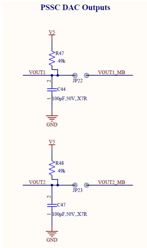
**Figure 11. VOUT1/VOUT2 Output Filtering**
