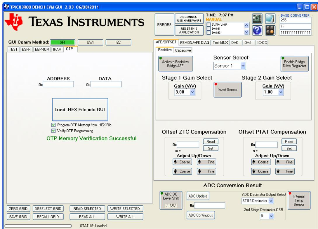
Figure 18. OTP Memory Successful Programming Verification
