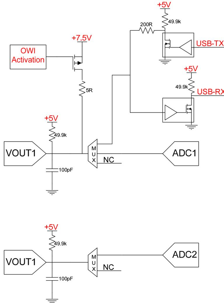
Figure 10. Simplified Block Diagram of PGA400-Q1 Output Circuitry
