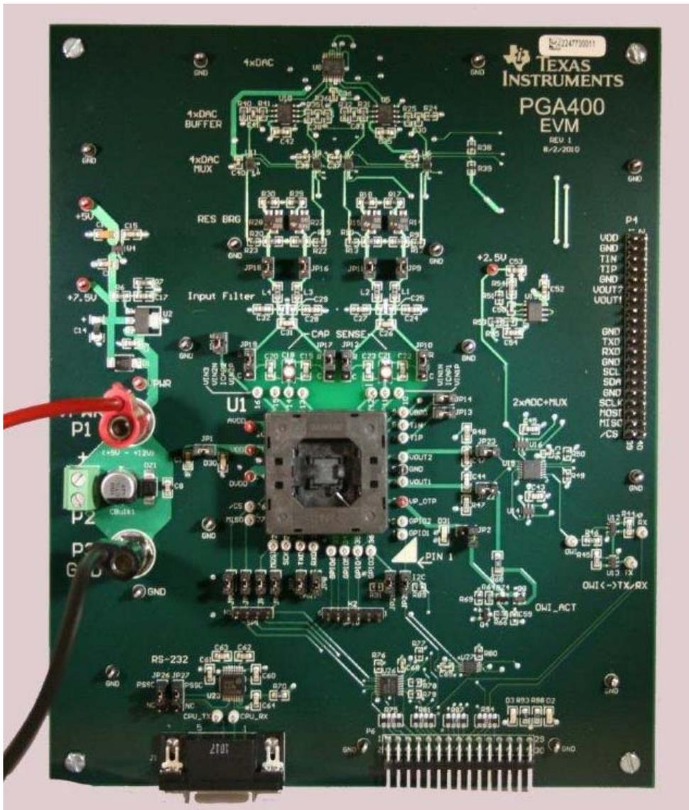
Figure 1. Minimum Power Connections to the PGA400-Q1 EVM
