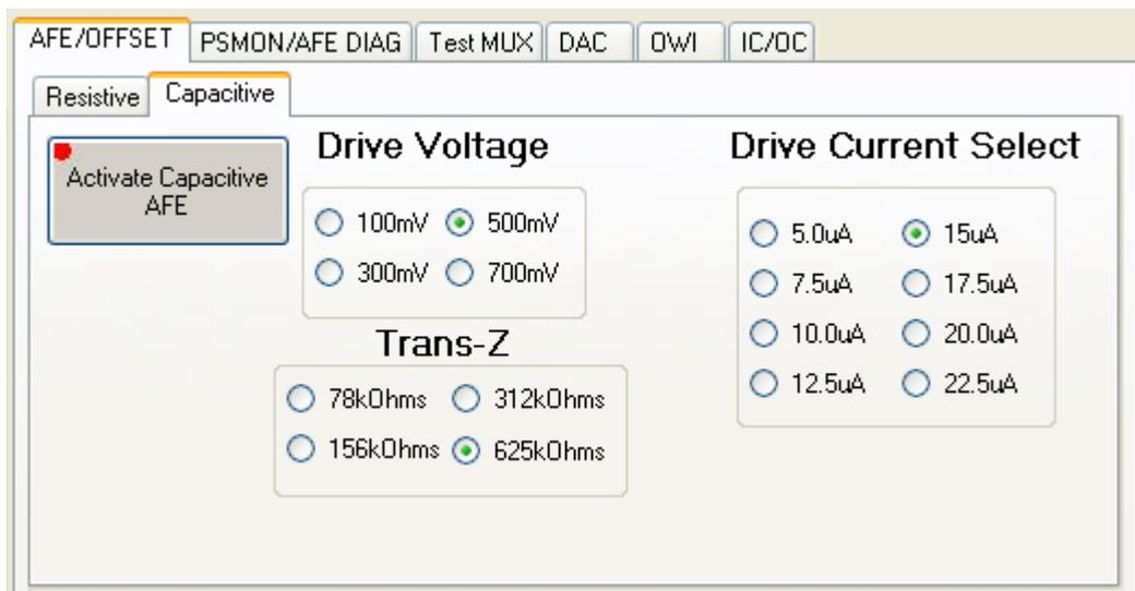
Figure 21. Capacitive AFE Tab
