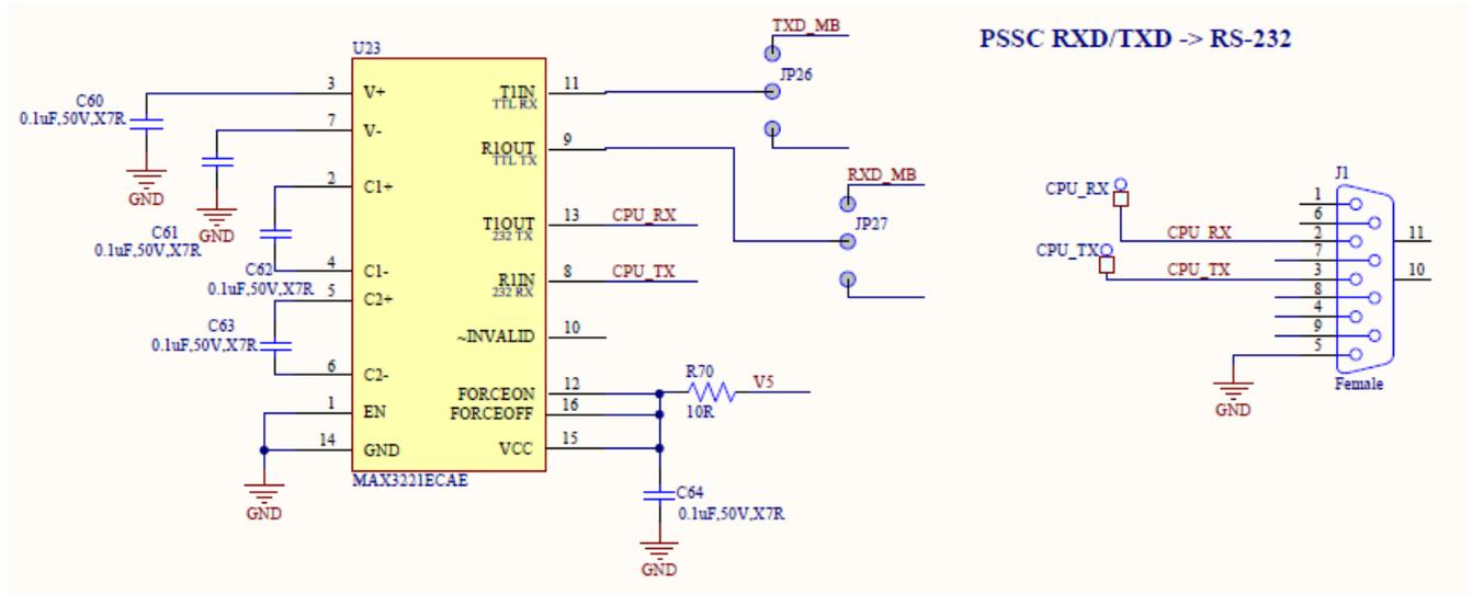
Figure 16. RS-232 Transceiver
