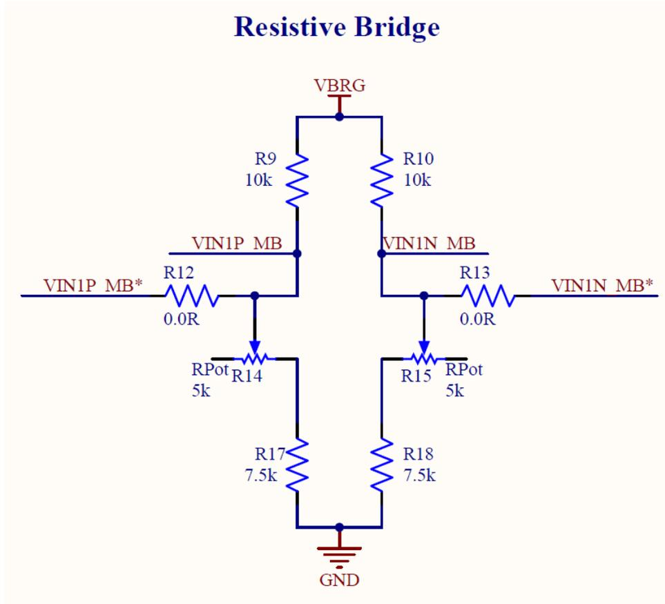
Figure 6. Channel 1 Resistive Bridge Sensor Simulator
