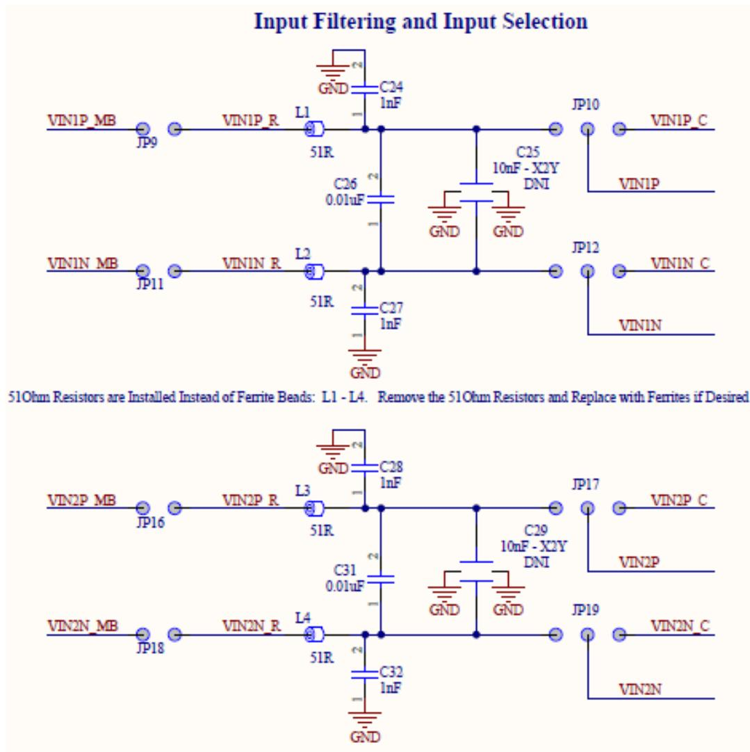
Figure 8. Input Filtering on the PGA400-Q1 EVM
