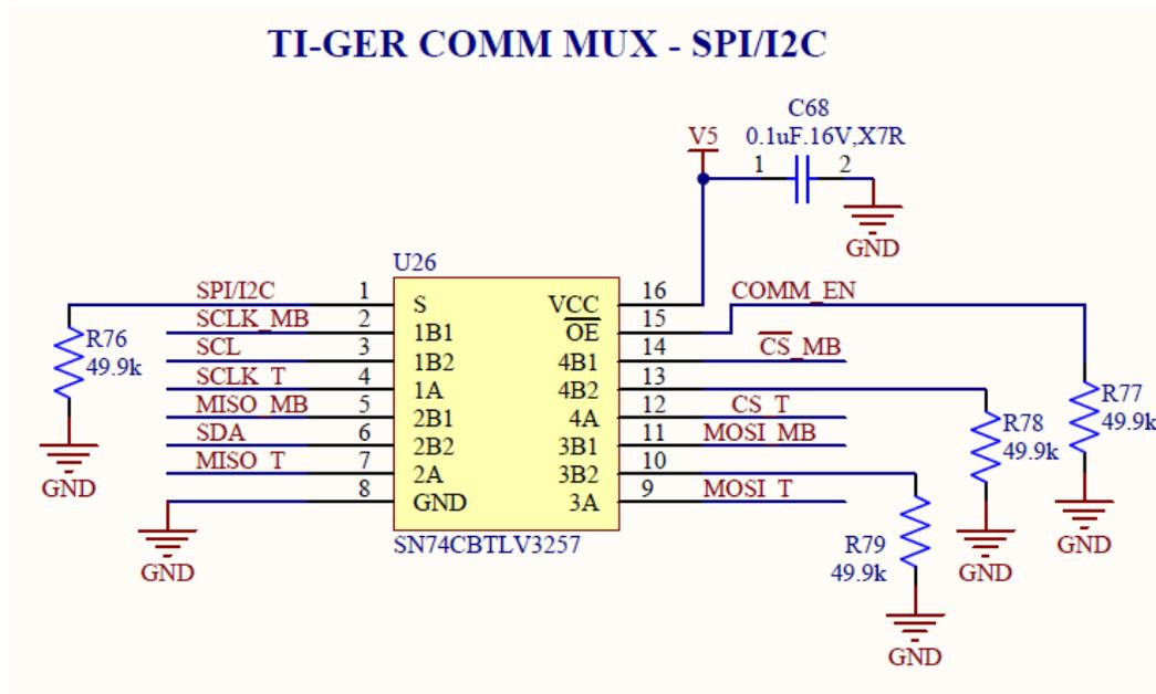
Figure 14. SPI/I2C Communication MUX
