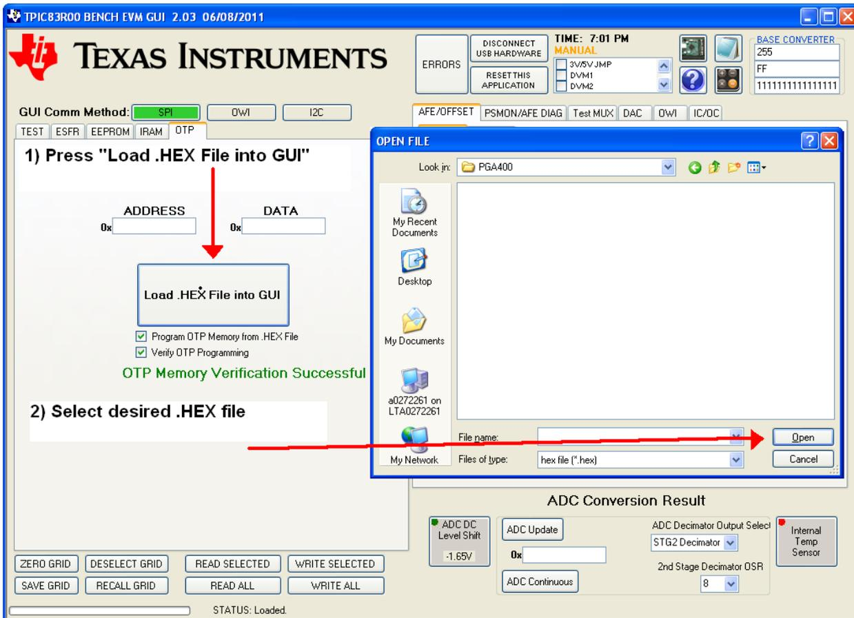
Figure 17. Loading a .HEX File into the GUI
