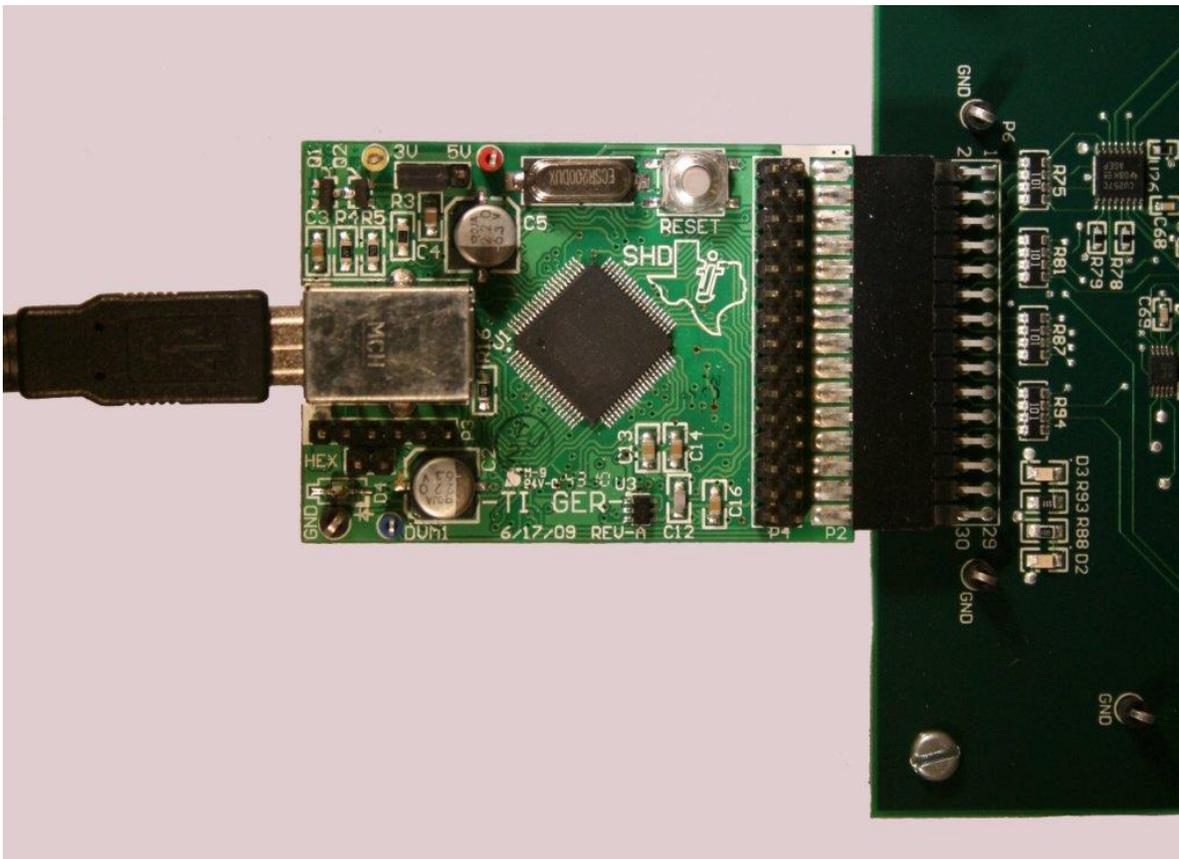
**Figure 3. Connecting the TI-GER USB Communication Board to the PGA400-Q1 EVM**
