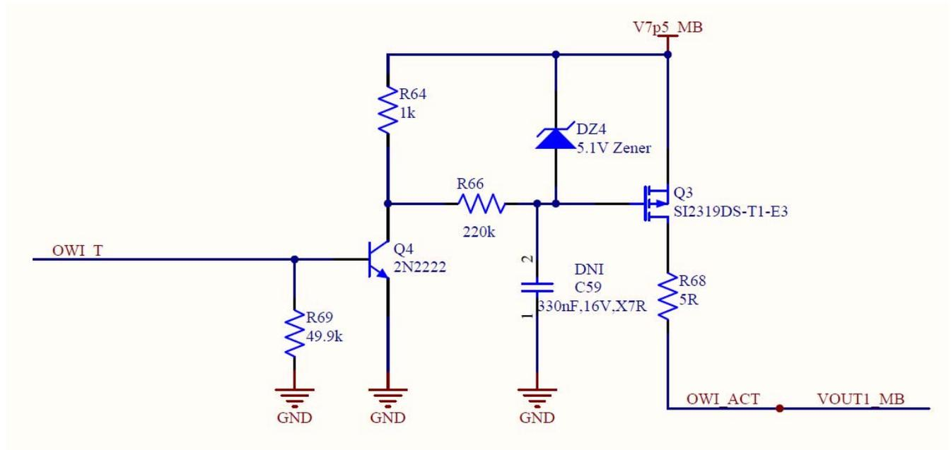
Figure 12. OWI Activation Circuit
