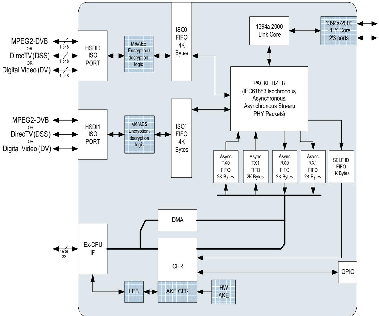
NOTE: Blocks with checked/shaded pattern are available only in selected versions of the device.
