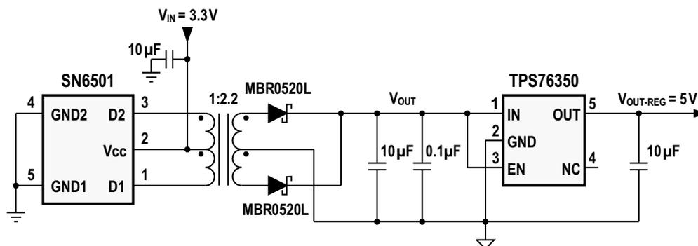
Figure 1. SN6501EVM Pinout and Functional Block Diagram
