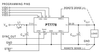
$\begin{array}{ll} C_{in} &= Required\ 2400\mu F\ electrolytic \\ C_{out} &= Required\ 330\mu F\ electrolytic \\ L1 &= Optional\ 1\mu H\ input\ choke \end{array}$
