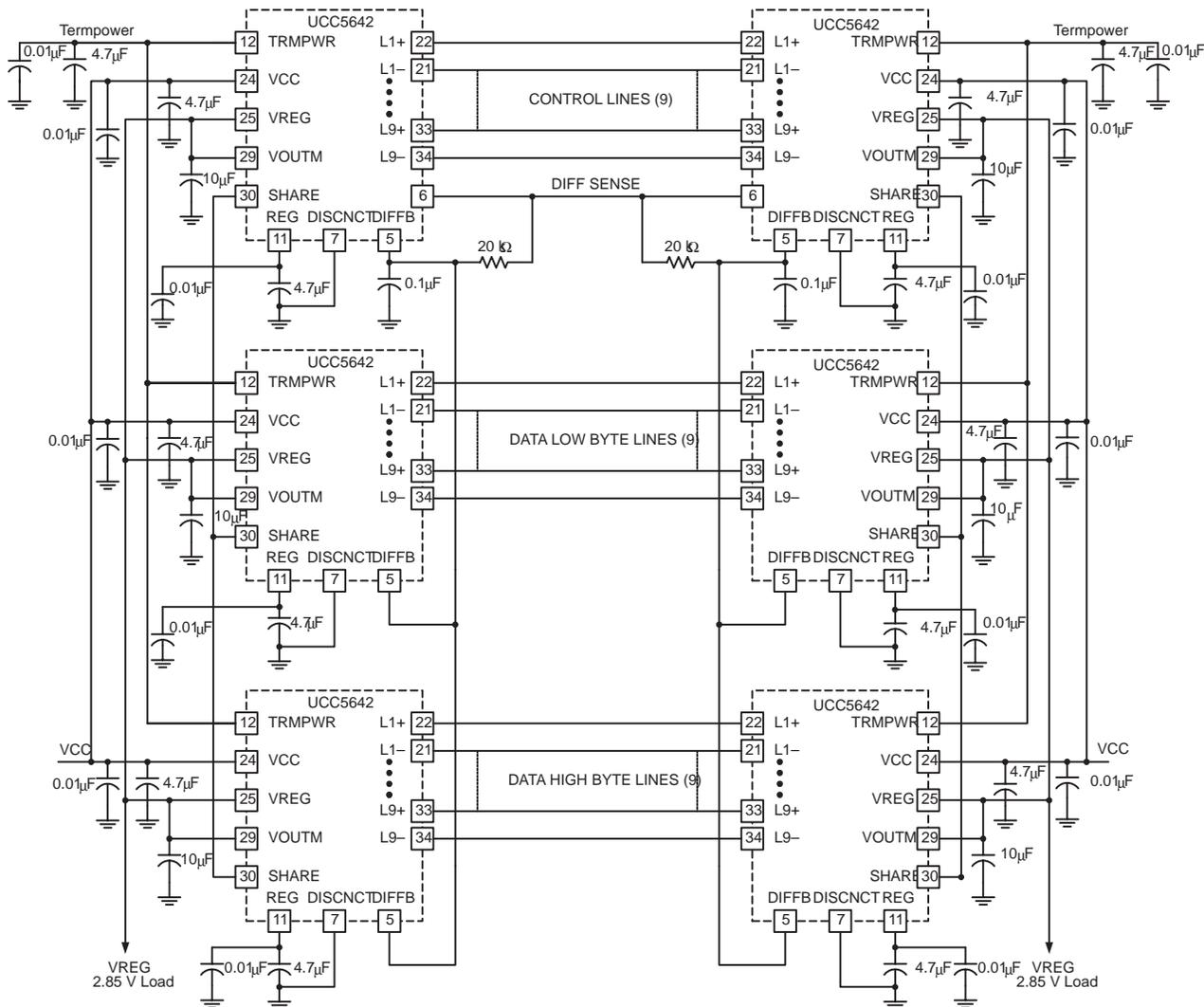
**Figure 1. Application Diagram**
