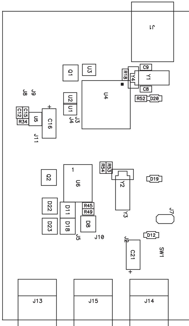
Figure 5. Component Placement 1
