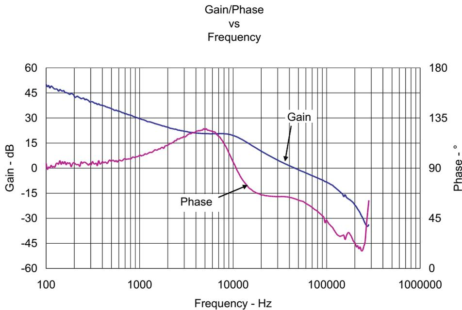
Figure 12. TPS40195EVM Bode Plot  $V_{IN} = 12\text{ V}$ ,  $I_{OUT} = 0\text{ A}$ ,
