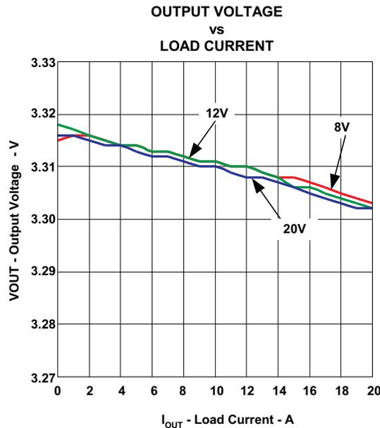
Figure 6. TPS40195EVM Line and Load Regulation  $V_{IN} = 8\text{ V to }20\text{ V}$ ,
