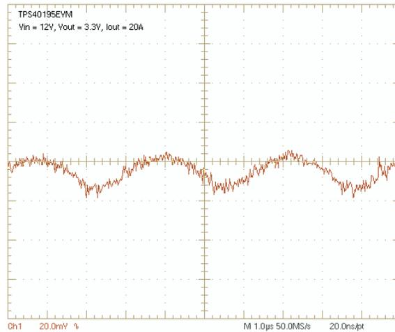
**Figure 8. TPS40195EVM Output Voltage Ripple**
