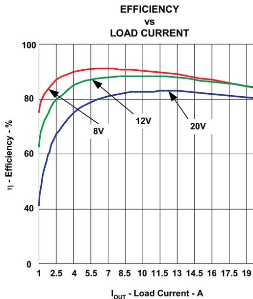
Figure 7. TPS40195EVM Efficiency  $V_{IN} = 8\text{ V to }20\text{ V}$ ,
