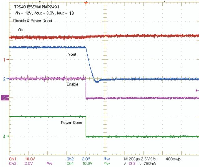
**Figure 13. TPS40195EVM Disable and Power Good,  $V_{IN} = 12V$ ,  $I_{OUT} = 10A$ , Ch1: TP1 ( $V_{IN}$ ), Ch2: TP5 ( $V_{OUT}$ ), Ch3: TP11 (ENABLE); Ch4: TP9 (Power Good)**
