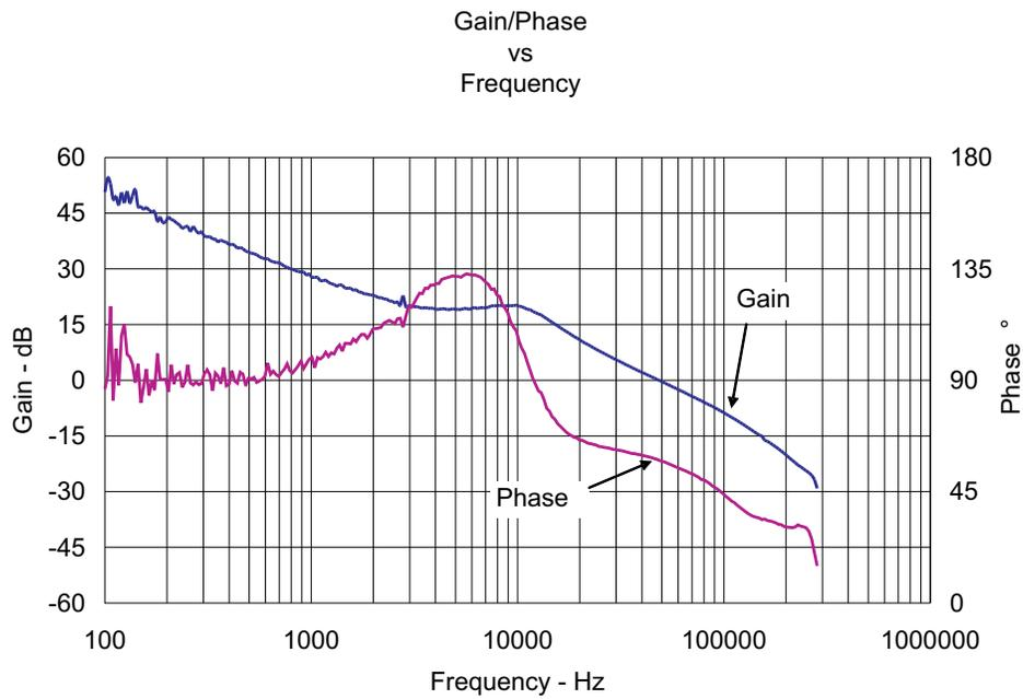
Figure 11. TPS40195EVM Bode Plot  $V_{IN} = 12\text{ V}$ ,  $I_{OUT} = 20\text{ A}$ ,
