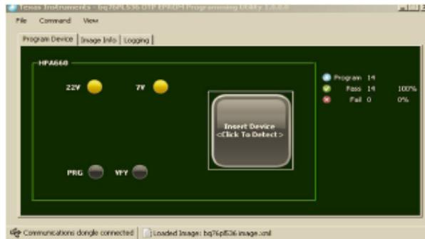
Figure 16. Completed EPROM Programming. Insert a New IC and Repeat From Step 5.
