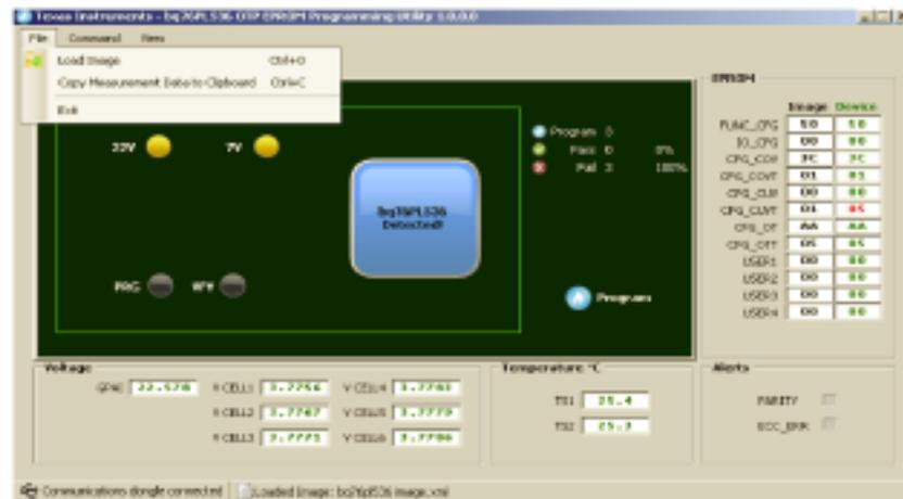
Figure 20. Copying Measurements Data to Clipboard
