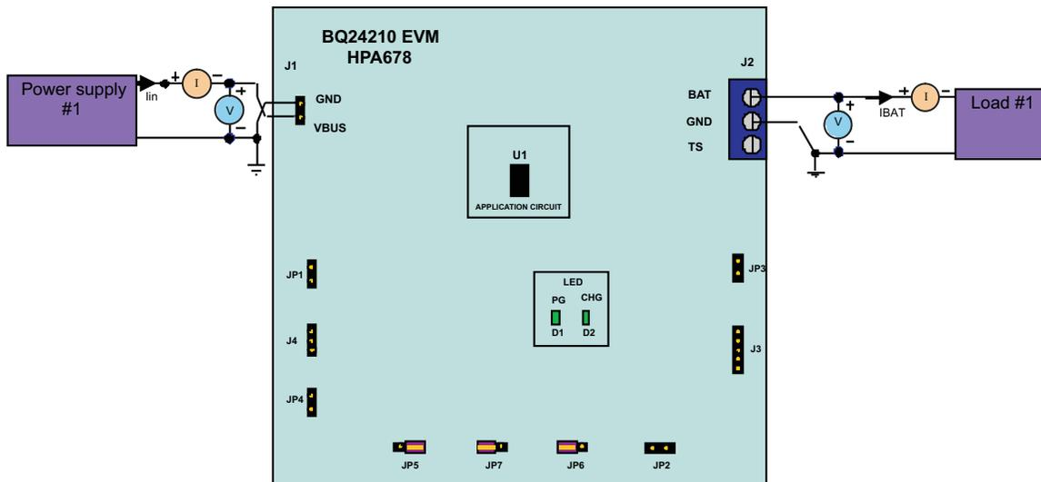
Figure 1. Original Test Setup for HPA678 (bq24210/2EVM)
